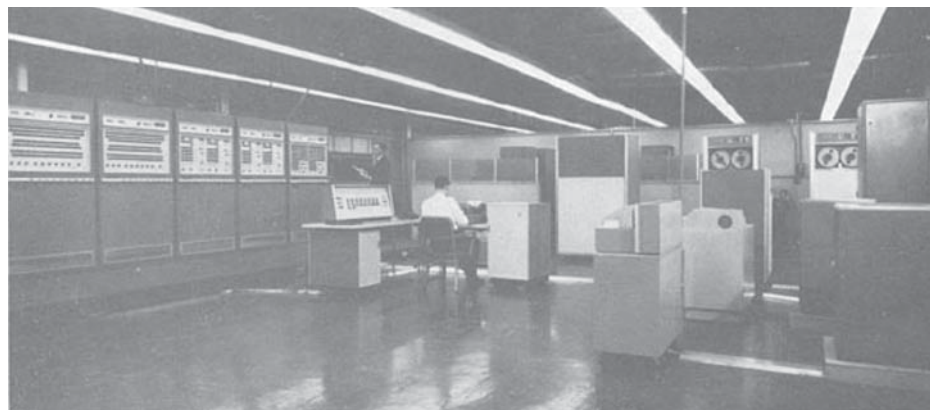
Figure 1.2 Photograph of Burroughs Corporation's D825 parallel computer [6]
