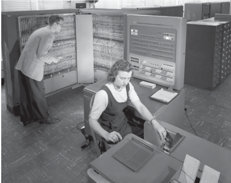
Figure 1.1 Photograph taken in 1957 at NASA featuring an IBM 704 computer, the first commercially available general-purpose computer with floating-point arithmetic hardware [4]
