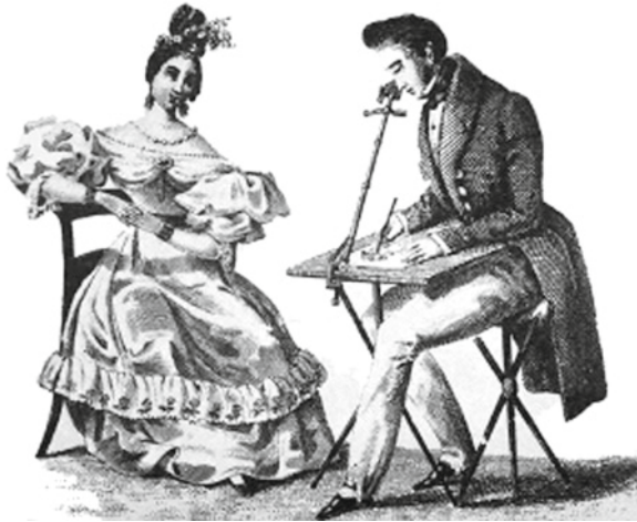
Fig. 3.1 An 1807 engraving of a camera lucida in use (Unknown artist. Wikimedia Commons. No known restrictions on publication)
