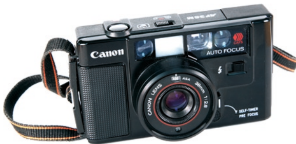
Fig. 4.8 The Canon AF-35M was named the Autoboy in Japan and Sure Shot in the US. Launched in November 1979, it was the world's first lens-shutter 35 mm autofocus camera 146 (© Olli Pitkänen and Risto Sarvas, 2010. Published with permission)
