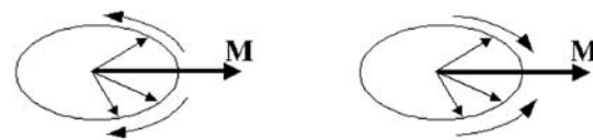
Gradient Echo technique: A gradient in the magnetic field causes the spins to lose phase coherence. Reversal of the gradient causes them to regain it.
