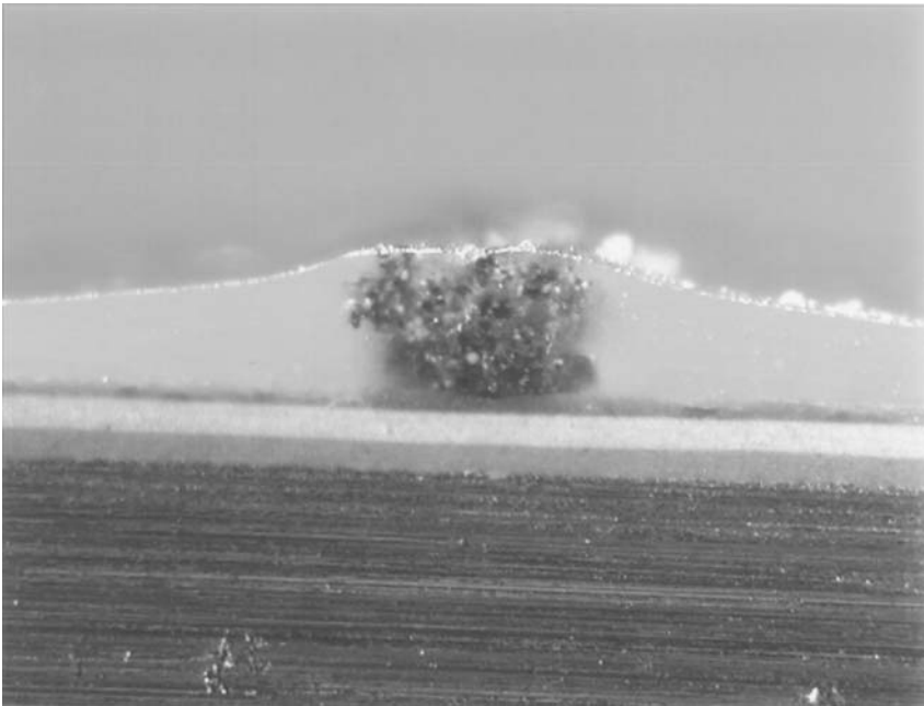
FIG. 18 Cross section showing a clump of basecoat overspray in a clearcoat.
