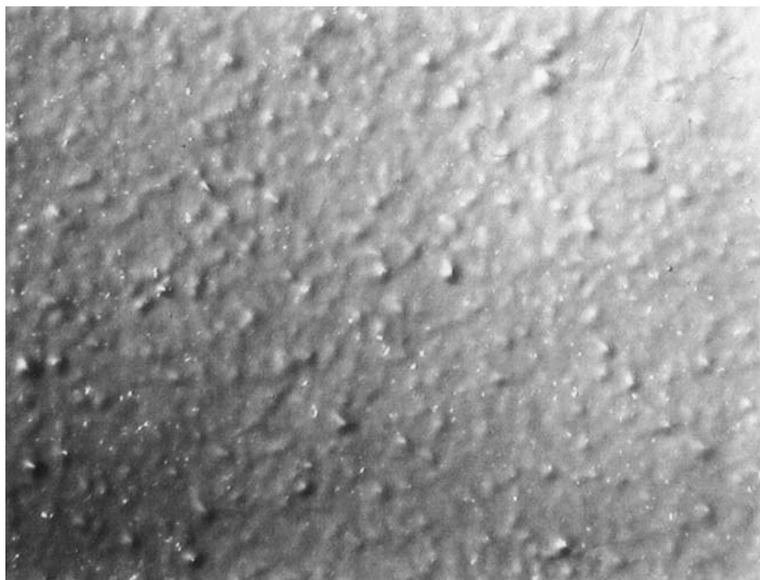
FIG. 12 Example of micropopping. Perhaps, microbumps is a more accurate description in this case. To the eye, the effect is one of fuzziness of reflections.
