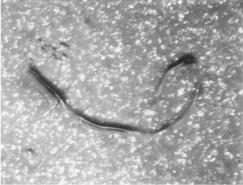
FIG. 14 Dirt—an example of a fiber.
