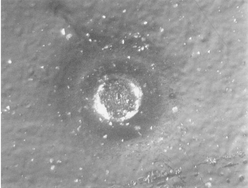
FIG. 10 Gassing from a plastic substrate. Note the hole in the center of the defect.
