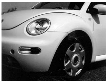
FIG. 14 2001 Volkswagen Beetle fender of PPO/PA.
