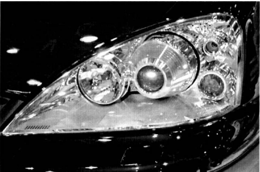
FIG. 12 Example of polycarbonate used in lens cover: 2001 Ford Mondeo headlight assembly with a PC lens cover and metallized reflector.
