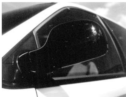
FIG. 13 Unpainted ASA/AES mirror housing.
