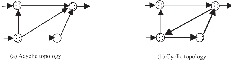
1.2 Illustration of (a) an acyclic graph and (b) a cyclic graph. The cycle in (b) is emphasized with thick lines.
