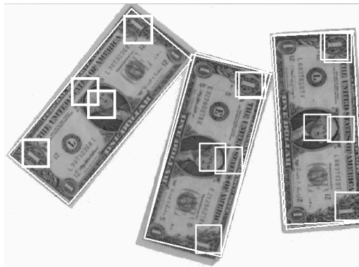
13.9 Money patterns detected by a hierarchical DBNN recognizer. The small boxes indicate the locations of the detected local currency texture features, and the large boxes show the locations of the money patterns. (With permission from S.Y. Kung, J. Taur, and S.H. Lin, Synergistic modeling and applications of hierarchical fuzzy neural networks, Proceedings of the IEEE , vol. 87, no. 9, pp. 1550–1574, 1999.)
