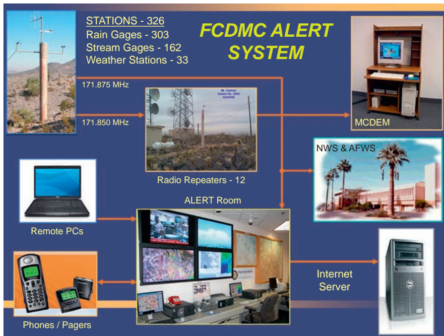
Plate 10 Flood early warning system for flood control district of Maricopa County (FCDMC) (Courtesy of FCDMC)
