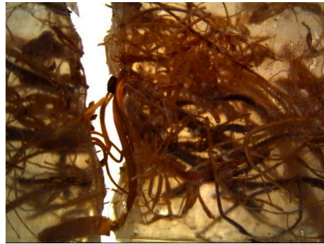
Fig. 2: Tensile failure of 3% untreated fiber reinforced in the epoxy matrix
