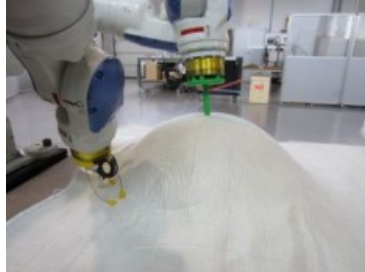
Figure 3: Automatic draping with self-developed tools (left) and robot simulation (right)
