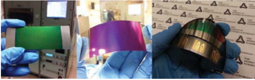
Figure 3.22 (a) Alumina coatings on stainless steel foil with different thickness values and (b) first prototype of flexible Stainless Steel/Mo/CIS/Ag-InS/ZnO/AZO-Ag-AZO/Ni/Al structure solar cells manufactured at TOBB University of Economics and Technology.
