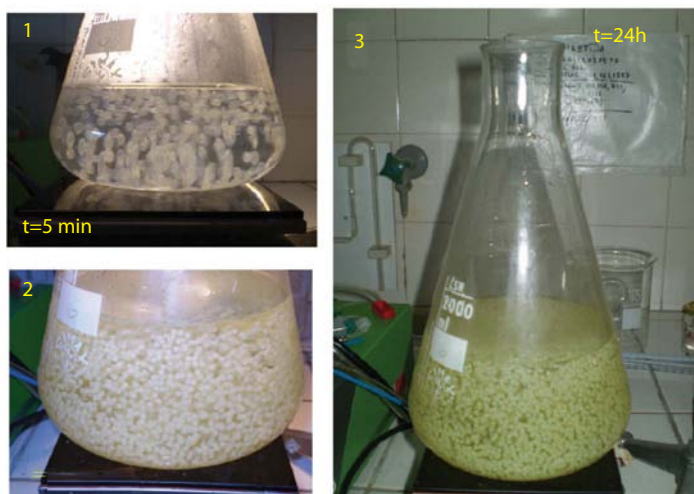
Figure 11.4 Photos for the synthesis of cross-linked chitosan microspheres in different time periods (the photos were taken during the synthesis in our laboratory) (General & Inorganic Chemical Technology, Aristotle University of Thessaloniki, Greece).
