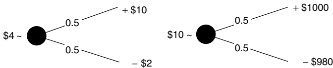
Figure 5.15 Despite the higher EMV of the right-hand bet most people would choose the bet on the left.
