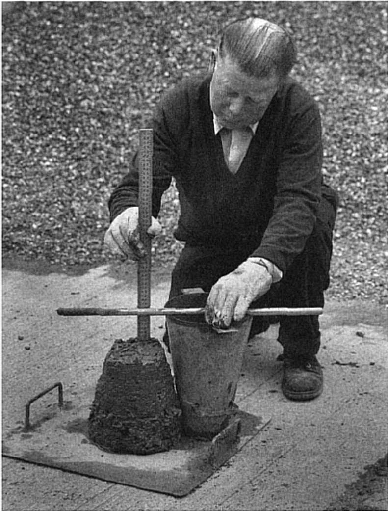
Figure 2.1 The slump test: measuring the slump. ( Photo courtesy of the British Cement Association ).
