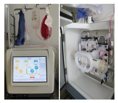
**Fig. 1** The Quantum Cell Expansion System. (a) Illustrates the workstation with the instrument touch screen and medium bag, cell inlet bag, and waste bag on the bag pole. (b) Shows the hollow fiber bioreactor, the peristaltic pumps, and valves
