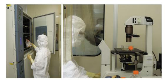
**Fig. 2** Media Fill Equipment. Equipment used in Media Fill runs, like  $CO_2$  incubators (a), Phase contrast microscope (b) etc., are the same as in cell manipulation production process
