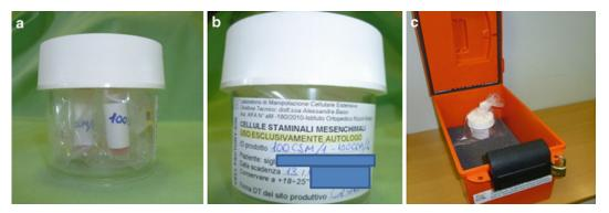
**Fig. 4** Final product packaging. The final cellular products is transferred into proper tubes (primary container, **a**), then put it into secondary sterile bags (secondary container, **a**). The product is then inserted in a plastic jar, properly labeled (**a** and **b**). For the shipment a container with lock is utilized (**c**)
