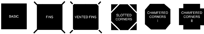
Figure 8-1. Aerodynamic modifications to a square building shape
