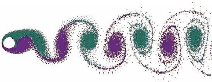
Figure 4.1 Kármán vortex street (Source: Wikipedia ( http://en.wikipedia.org/wiki/File:Vortex-street-animation.gif ), Reproduced with permission from original author: Cesareo de La Rosa Siqueira).
