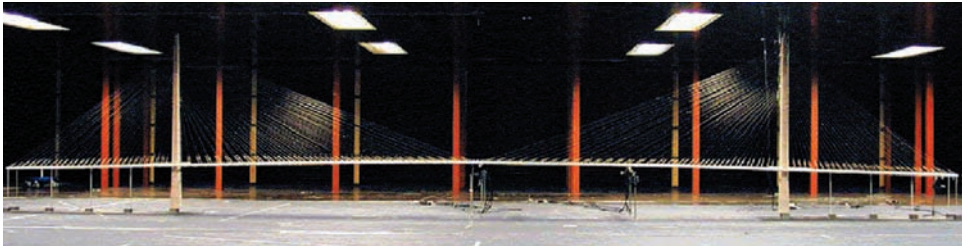
Figure 7.20 Full aeroelastic model test of Stonecutters Bridge (Reproduced with permission from Dr. Michael Hui).
