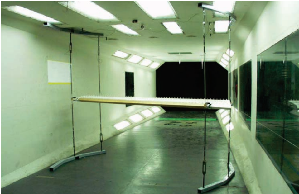
Figure 10.13 Installation of dynamic sectional model in TJ-2 wind tunnel ( \bar{\beta} = 31^\circ ) (from [28]) (Reproduced with permission from Elsevier).
