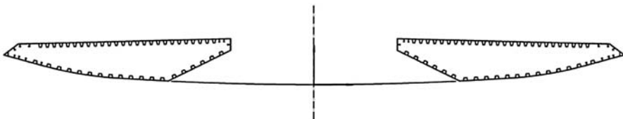
Figure 3.11 A typical cross-section of longitudinal steel girders.
