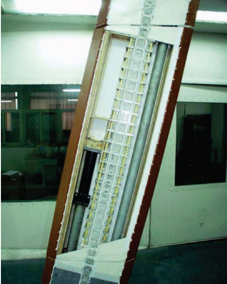
Figure 10.10 Force balance and steel pipes in model (from [27]) (Reproduced with permission from Elsevier).
