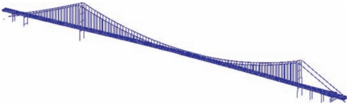
Figure 3.8 Multi-scale finite element model of the Tsing Ma Bridge (from [12]) (Reproduced with permission from Taylor & Francis).
