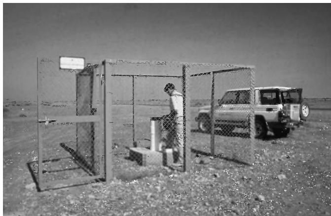
Figure 3.12 An observation borehole located near to an artificial recharge dam in northern Oman. Photo by Bruce Misstear
