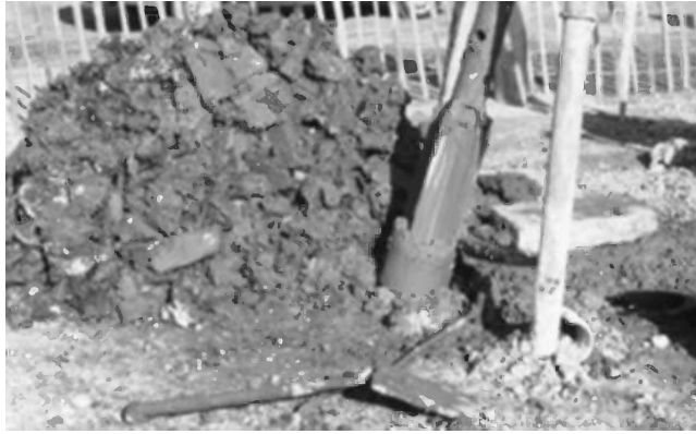
Figure 6.4 A clay cutter, used to extract samples of cohesive sediments encountered during cable-tool percussion drilling. Photo by Bruce Misteat
