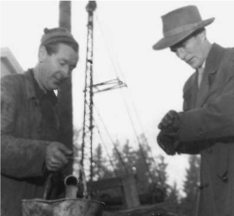
Figure 7.6 The Norwegian hydrogeologist Steinar Skjeseth uses a watch and bucket of known capacity to determine the yield from a pumping test of a well. After Banks and Robins (2002) and reproduced by permission of Norges geologiske undersøkelse (Geological Survey of Norway)
