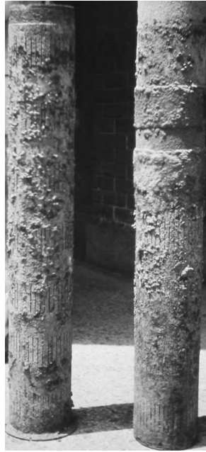
Figure 9.1 Encrusted well screens, Pakistan. The characteristic iron oxide 'tubercles' are visible on the surface of these steel screens. Photo reproduced by permission of Paul Ashley, Mott MacDonald Ltd
