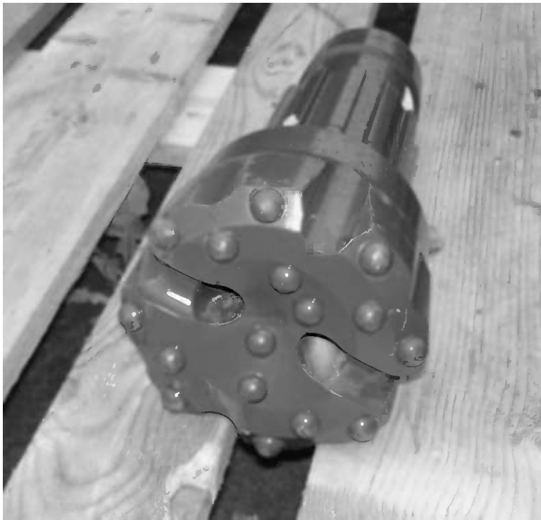
Figure 5.16 Button bit used for DTH hammer drilling. Photo by Bruce Misstear
