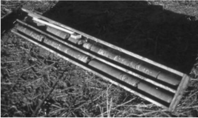
Figure 6.11 Storage of newly extracted cores in a core-box, landfill site, England. Photo by Bruce Misstear
