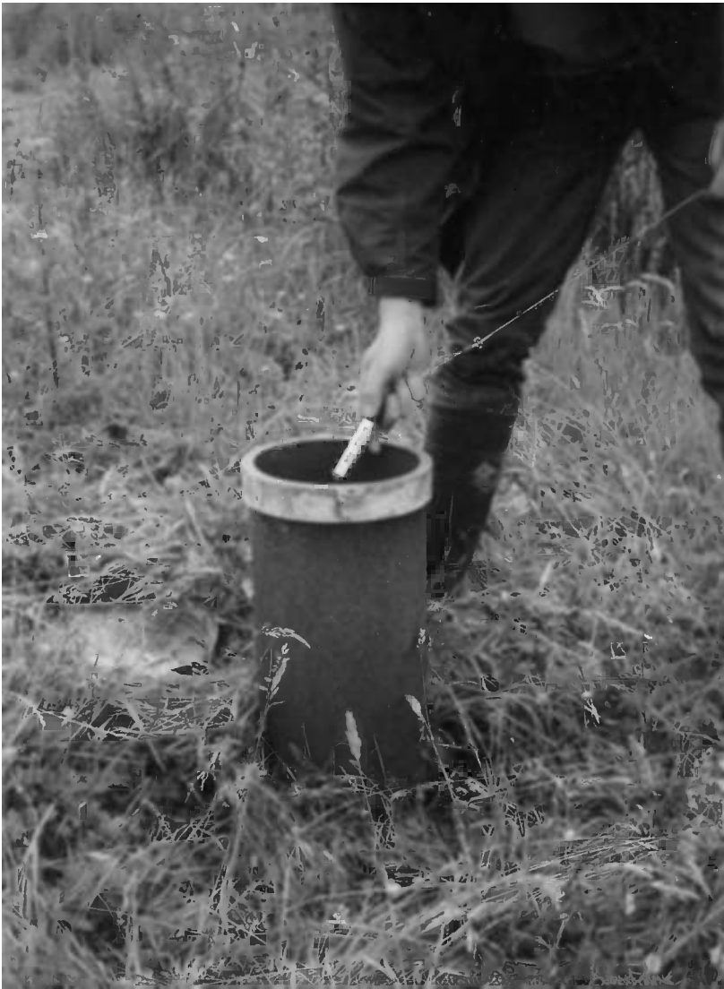
Figure 2.19 Small water level monitoring unit (incorporating pressure transducer, power source and data logger) being installed in an observation borehole in County Monaghan, Ireland. Photo by Bruce Misstear
