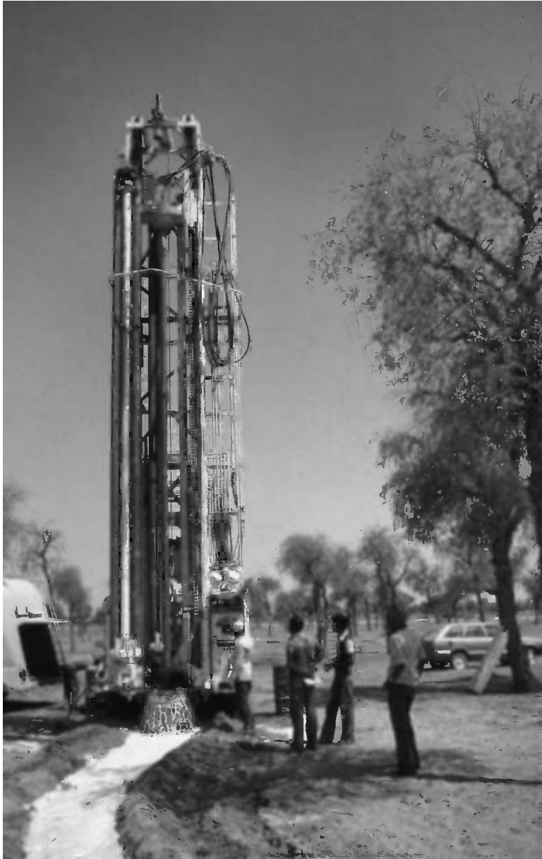
Figure 5.8 Air-foam drilling using a top-drive rotary rig, northern Oman. Photo by Bruce Misstear
