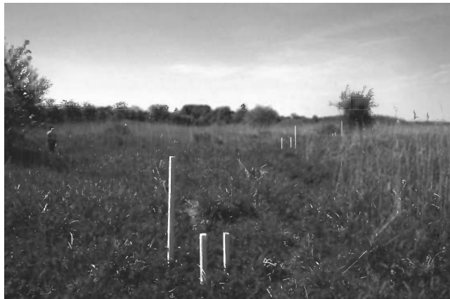
Figure 8.16 Clusters of piezometers at Pollardstown Fen, Ireland. Photo by Bruce Misstear
