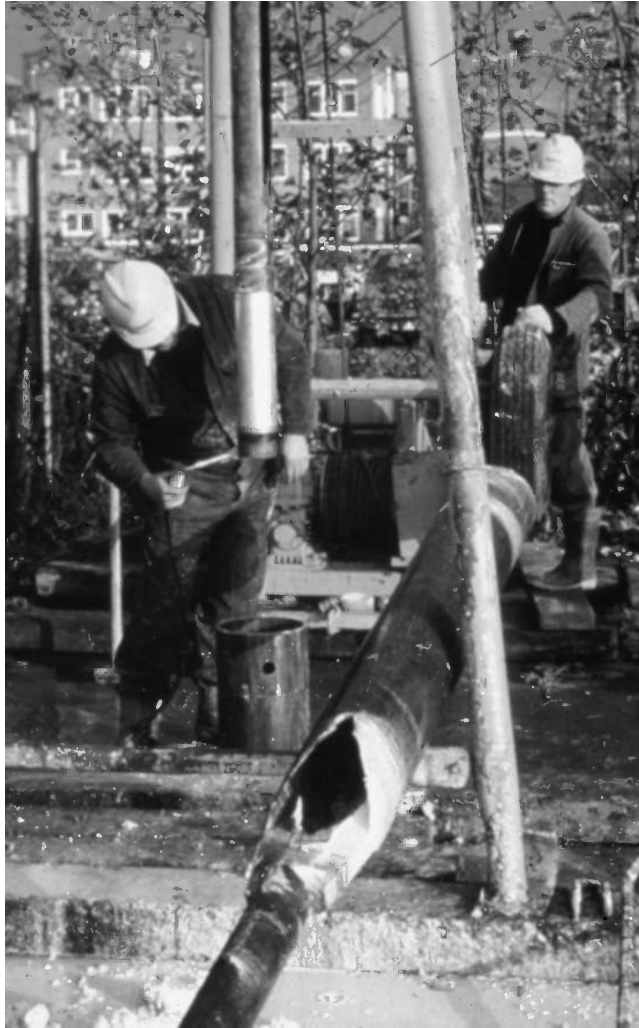
Figure 6.9 Flame cleaning of U100 tube sampler during an investigation of trace organic pollution, UK. Reproduced by permission of Paul Ashley, Mott MacDonald Ltd
