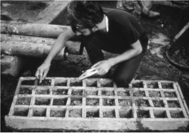
Figure 6.6 Disturbed formation samples being stored in sequential order of depth on site in a compartmentalized sample box. Reproduced by permission of Paul Ashley, Mott MacDonald Ltd
