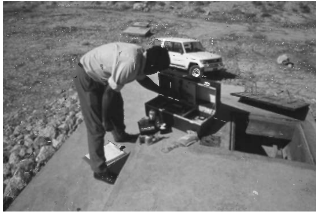
Figure 8.3 Portable water testing kits being used in Muscat. Photo by Bruce Mistear
