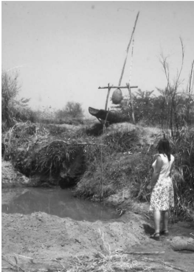
Figure 3.22 Shaduf used for lifting water from a temporary well in a dry river bed to an irrigated field beside the river bank, northern Nigeria. Photo by Bruce Misstear
