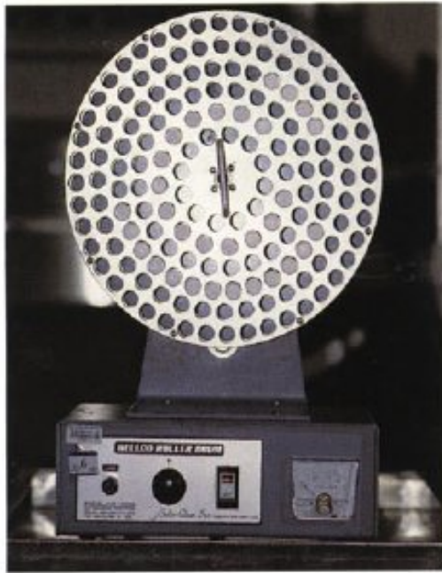
16-3 Roller drum (Bellco Glass, Inc., Vineland, N.J.). This instrument holds, and continuously rotates, tubes containing cell lines. The drum is placed inside an incubator at 33°–37°C. The holder containing the tubes can be removed from the incubator so that the tubes can be checked for CPE. This apparatus is most frequently used for culturing respiratory specimens for viruses such as influenza and parainfluenza.
