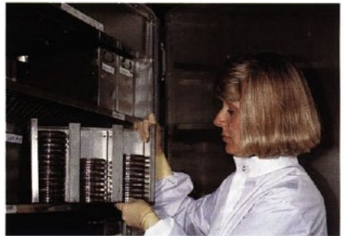
3-30 Media should be incubated as soon as possible after inoculation. As shown here, inoculated media is arranged in an orderly manner to minimize errors and avoid contamination.
