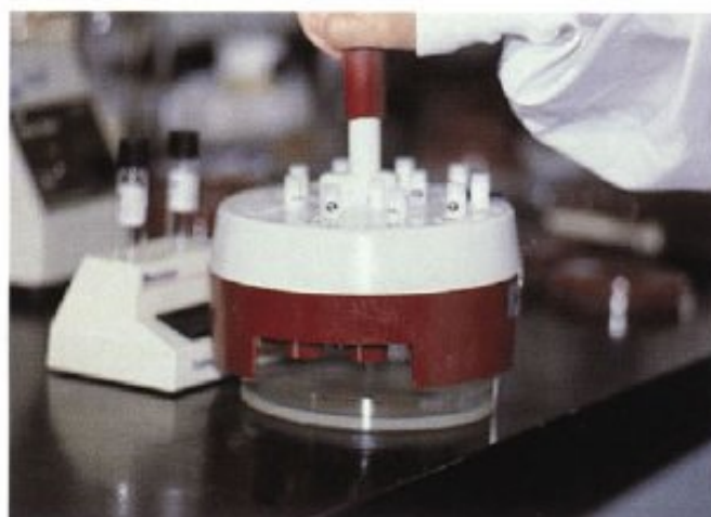
13-4 Disk diffusion method—application of disks. Disks are applied to the agar surface using a dispenser. No more than 12 disks should be placed on a 150 mm plate. A disk should not be relocated once it has made contact with the agar surface because antimicrobial diffusion begins immediately. Agar plates must be incubated within 15 minutes of disk application.
