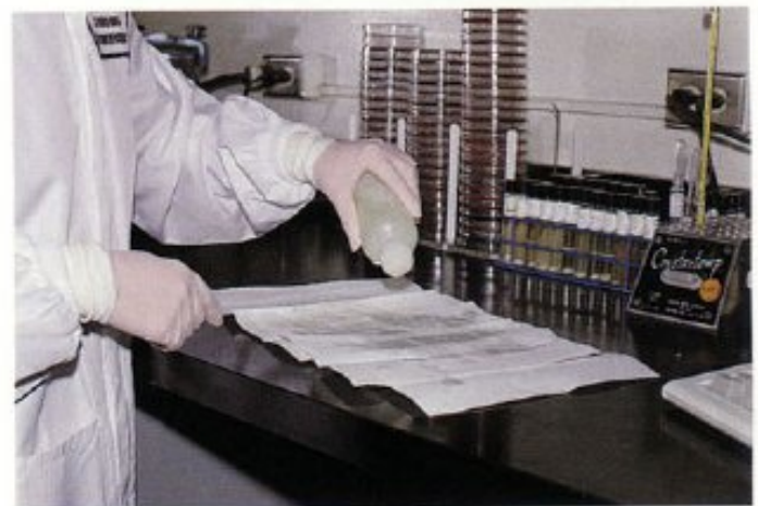
1-15 Paper towels should be placed on the contaminated work surface and soaked with diluted household bleach immediately after a spill and at the end of each shift.
