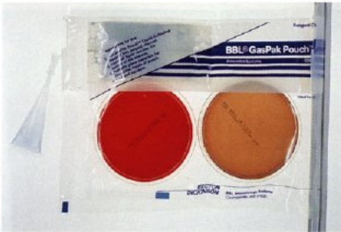
3-34 The GasPak anaerobic pouch (Becton Dickinson Microbiology Systems, Cockeysville, Md.) is based on the same principle. The bag is oxygen impermeable, and the system contains its own gas-generating kit and cold catalyst.
