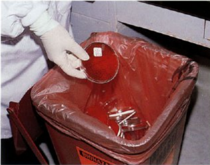
1-17 Agar plates are discarded in a properly labeled container with a lid.
