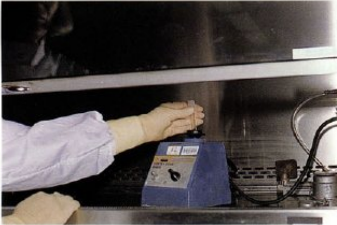
1-26 Tightly sealed containers should be vortexed in a BSC only. The tube should then be inverted to reabsorb aerosolized particles. A 30-minute wait before opening the tube avoids aerosol creation, especially when mycobacteria are being handled.
