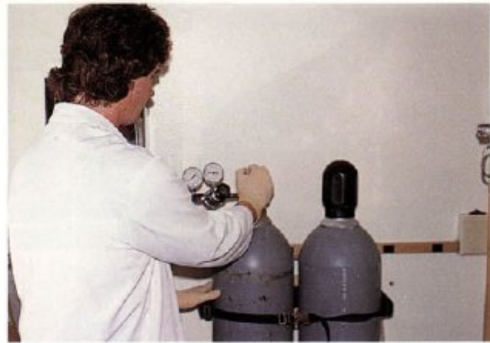
1-27 All gas tanks should be secured in place by a holding device.
