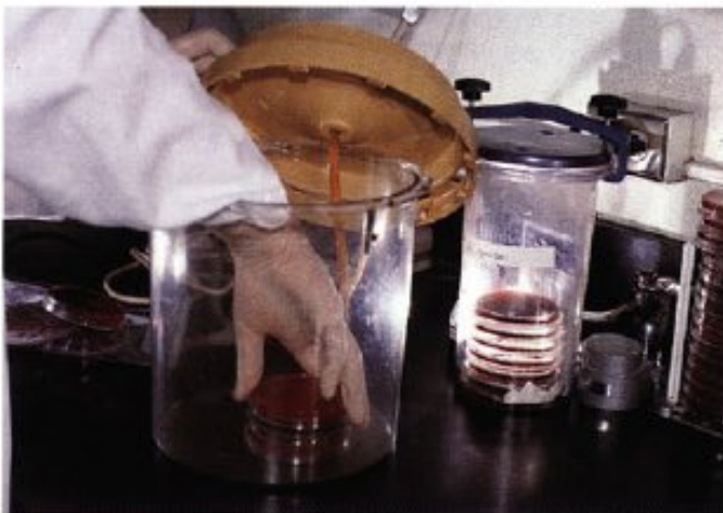
3-31 Prereduced anaerobic plates can be held in an anaerobic holding jar for a short time before and after inoculation.
