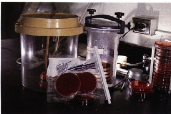
3-32 An anaerobic atmosphere can also be created in an anaerobic pouch that holds only two plates or in an anaerobic jar for three or more plates.
