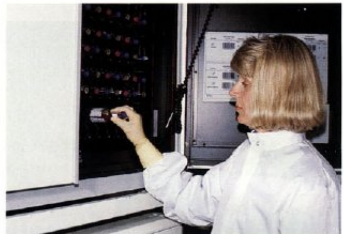
3-37 The technologist is placing a blood culture bottle into the BACTEC 9240 Fluorescent automated blood culture system (Becton Dickinson Diagnostic Instrument Systems, Sparks, Md.). Each bottle is entered into a cell of the incubator and monitored every 10 minutes by a photocell feedback system to a computer.
