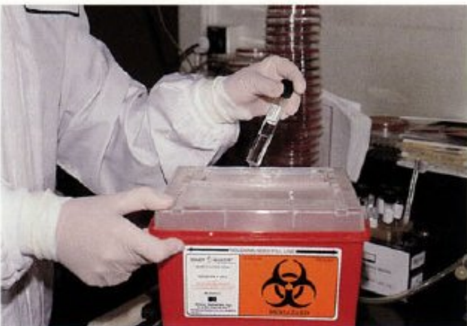
1-19 Glass tubes containing human samples are also discarded into hard-sided, puncture-proof containers.
