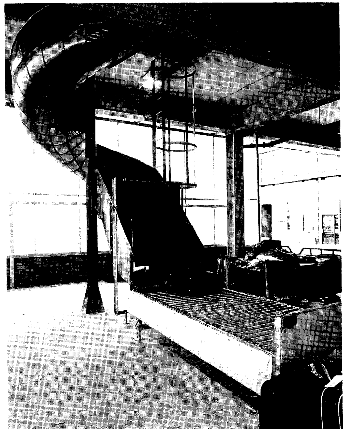
20.5 Gate baggage drop at London Heathrow Terminal 1. Figures 20.3–20.5 courtesy of Messrs Logan Fenamc.
