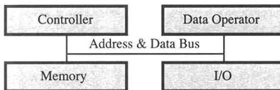
Figure 1.1. Simplified Computer Structure
