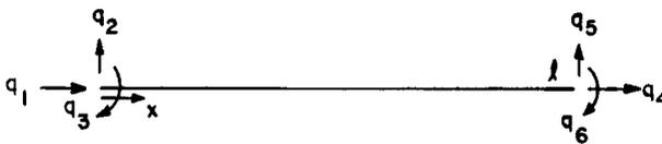
Fig. 1.1.1 Planar beam element.
