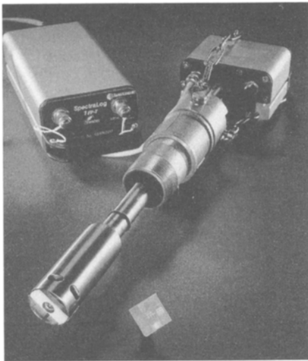
SpectraCense continuous on-line water quality monitoring apparatus for measuring, recording, and transmitting - pH, conductivity, dissolved oxygen, chlorine or free residual chlorine, turbidity and colour. (Manufacturers: Biwater SpectraScan, Waterlooville, Hants, UK)
