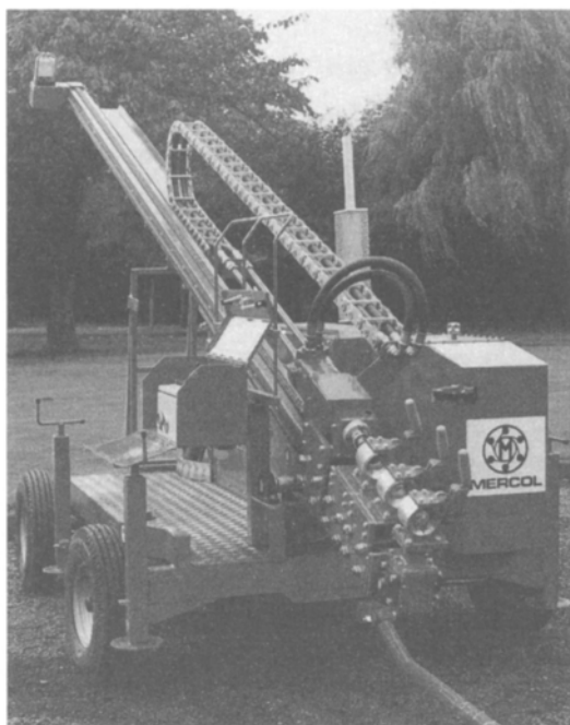
(Left) Mercol pipe cleaning equipment and (right) epoxy resin lining machine. (Mercol Products Ltd., Bolsover, Chesterfield, UK)
