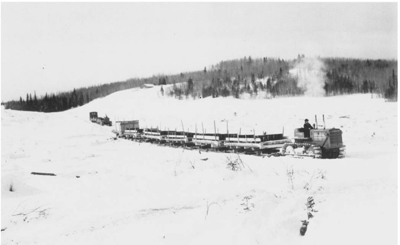
A Starways International tractor train plows through the winter bush in 1941 from Hudson to the Pickle Crow Mine. Note caboose at tail end.
