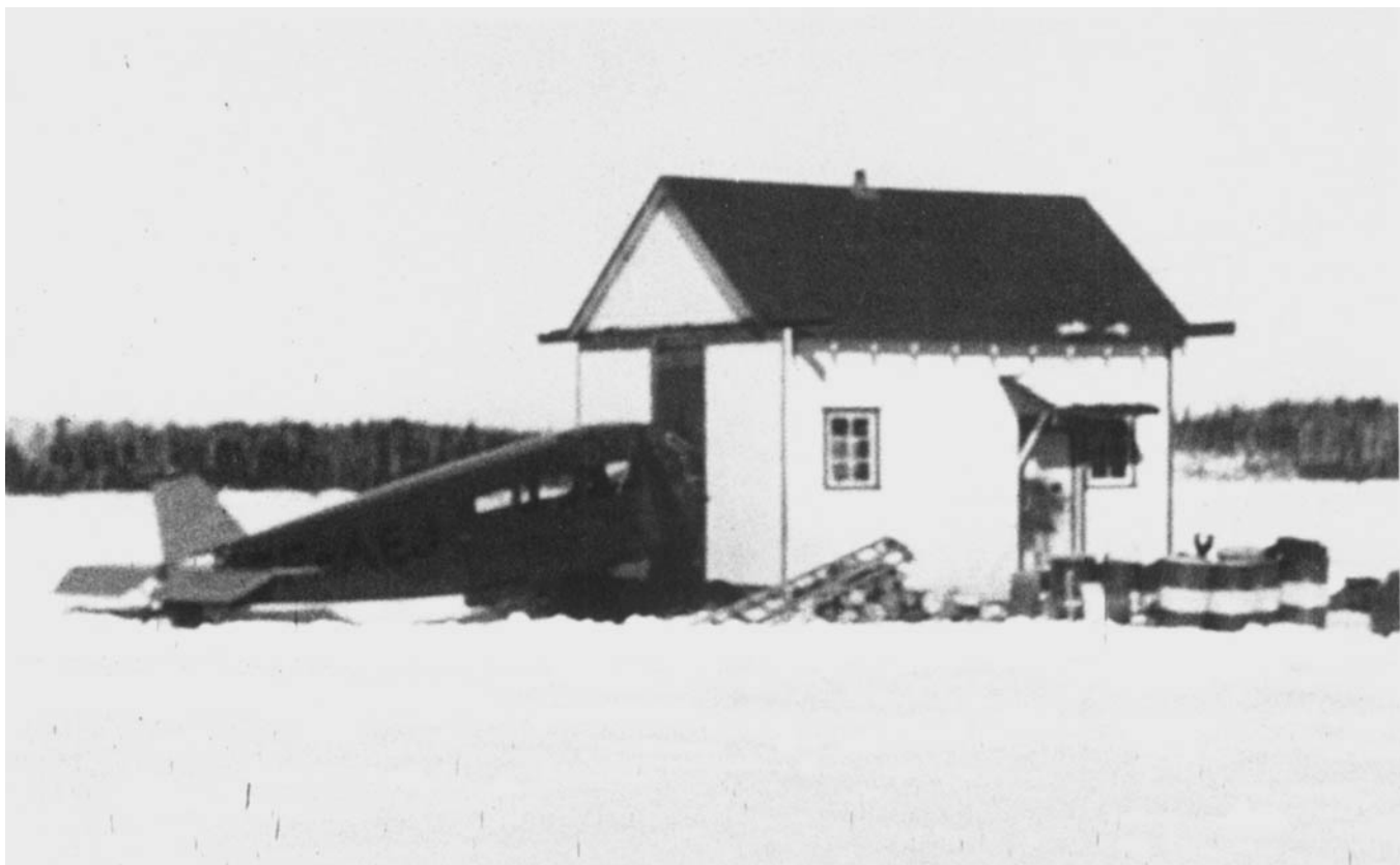
A portable nose hangar, mounted on runners for easy movement, was devised by bush pilot Harold (Doc) Oaks; having its nose warmed is a Travelair CFA EJJ.
