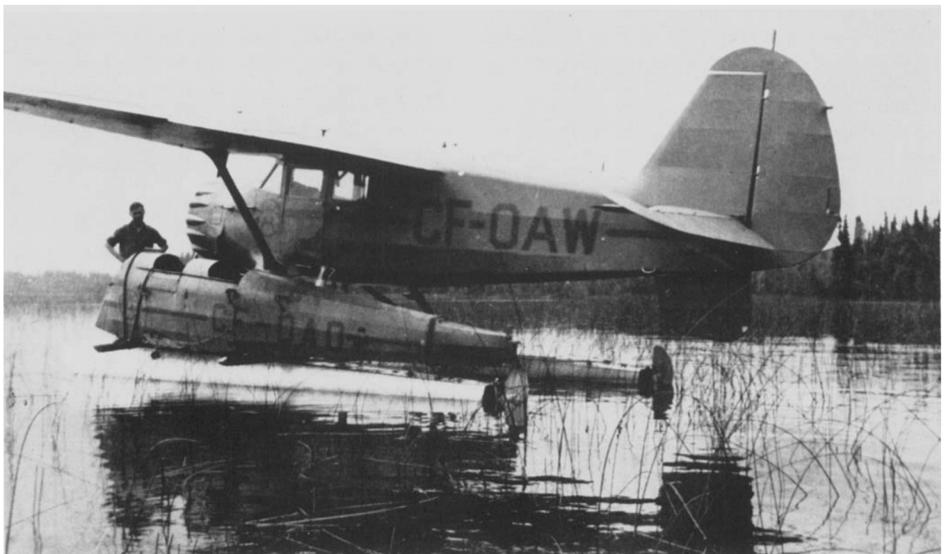
This Stinson OAW carries as cargo the entire fuselage of a salvaged Gypsy Moth lashed to its floats.
