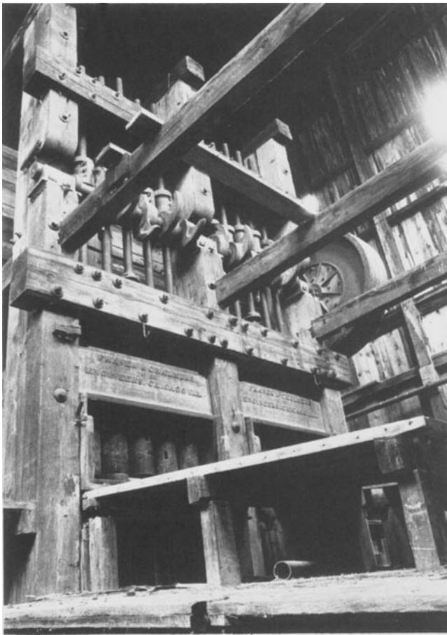
This complex stamping mill, with its imposing wooden fly wheel and heavy frame which turned a long iron cam shaft, used to operate like a sophisticated version of a druggist's mortar and pestle, liberating gold from the waste rock at the Detola Mine near Dryden.
