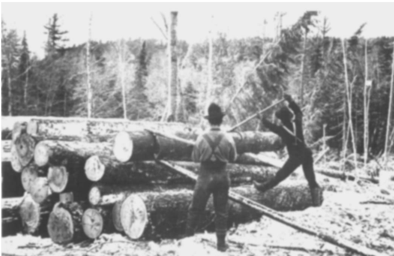
A cant hook — which to a layman looks like a stick with a hook hanging on it — was an effective tool for building a skidway, or storage pile of logs. The pair
