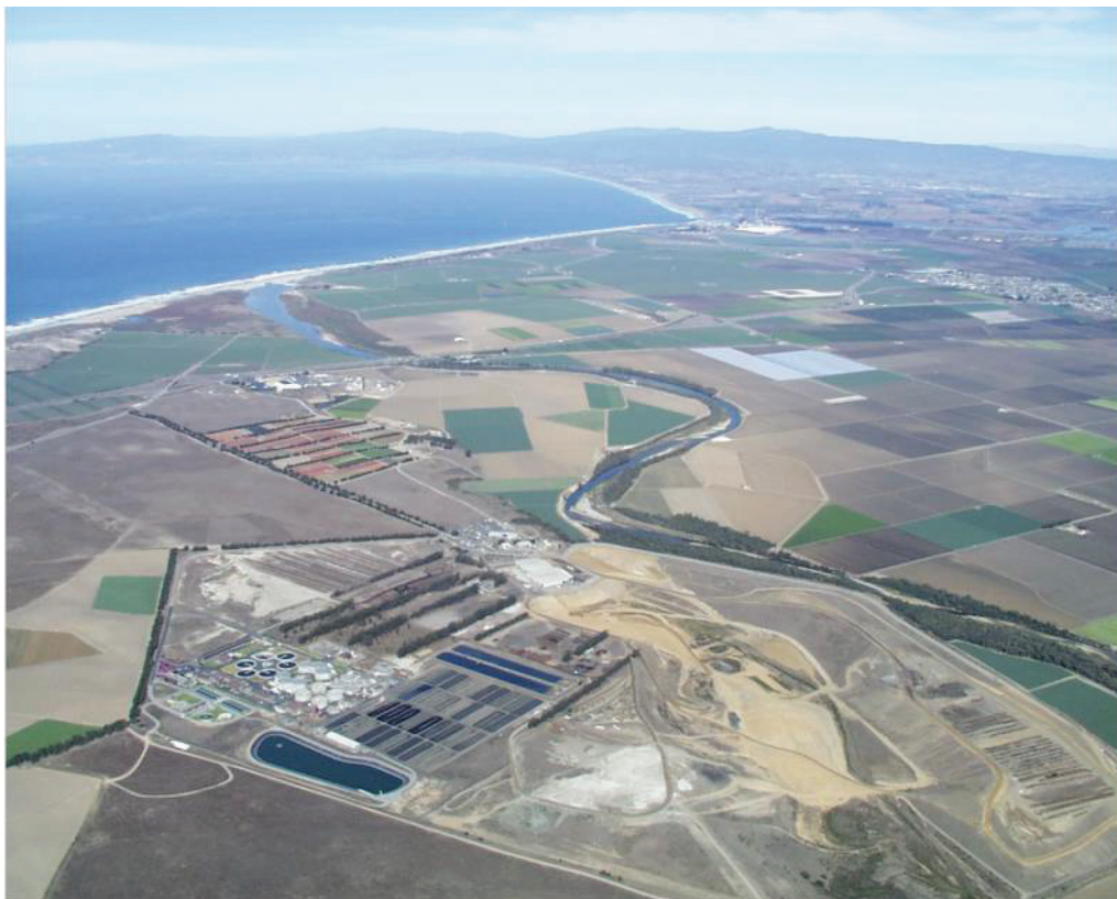
The Salinas Valley Reclamation Project in Monterey, California, which provides reclaimed water to area farms, thereby reducing seawater intrusion caused by overpumping the region's aquifers.
