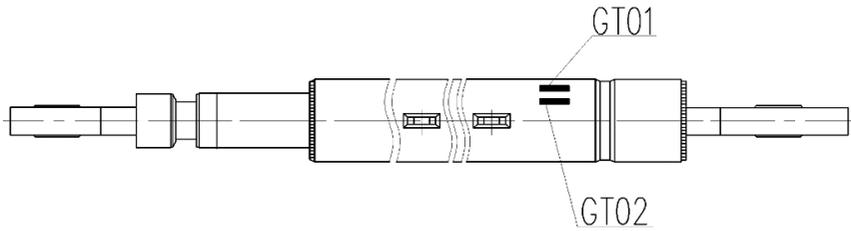
Figure 28. Strain and deformation measurement for hydraulic component.
