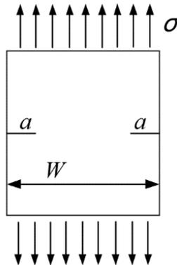
Figure 15. Double edge crack problem.
