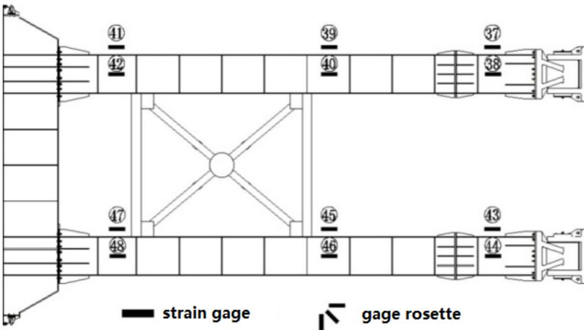
Figure 20. Measurement locations on lower beams.
