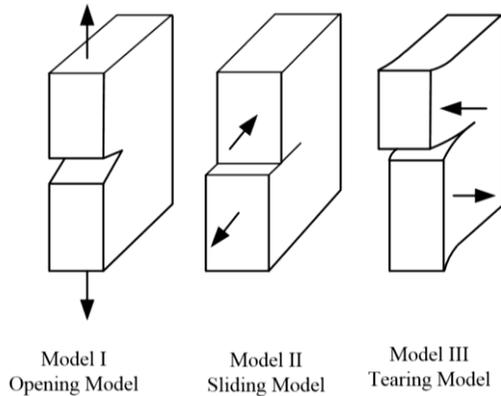
Figure 13. Fracture modes of crack problems.
