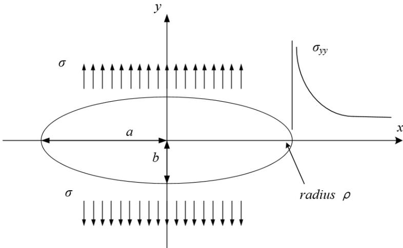
Figure 12. The elliptical hole problem.
