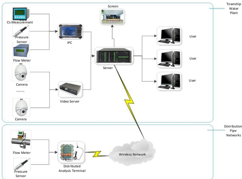
Figure 33. System architectures for water management in rural areas.
