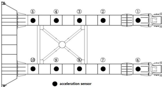
Figure 25. Locations for acceleration sensors on upper beams.
