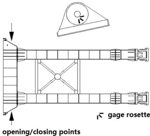
Figure 27. Measurement points for the opening/closing components.
