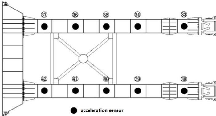
Figure 26. Locations for acceleration sensors on lower beams.
