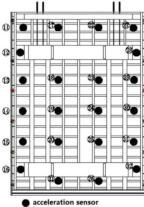
Figure 24. Locations for acceleration sensors on arc plate.
