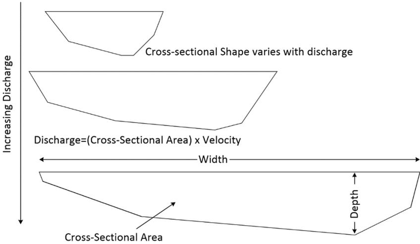
Figure 6. Relationship between river bed profile and discharge.
