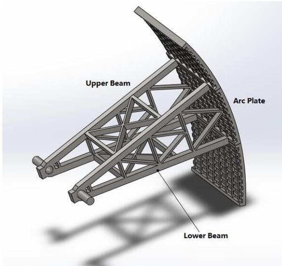
Figure 18. 3D plot of the mechanical structure of water gate system.
