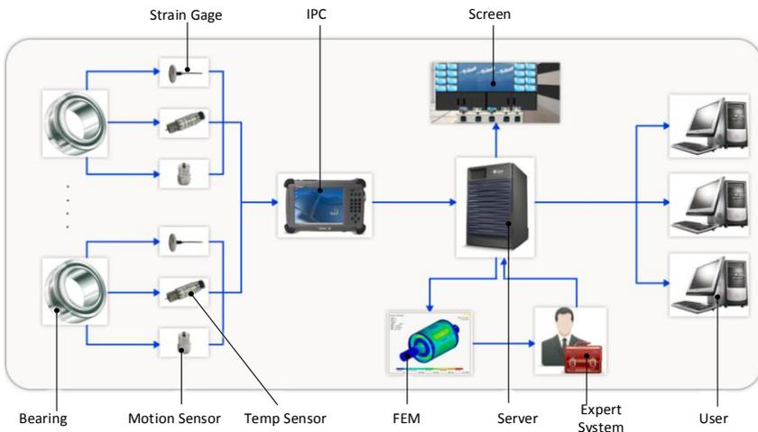
Figure 17. Architecture of safety management system for water gate system.
