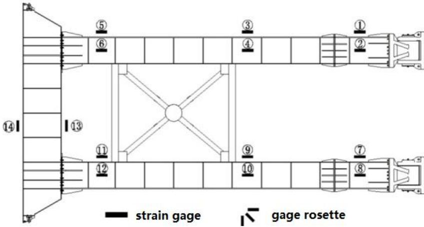
Figure 19. Measurement locations on upper beams.
