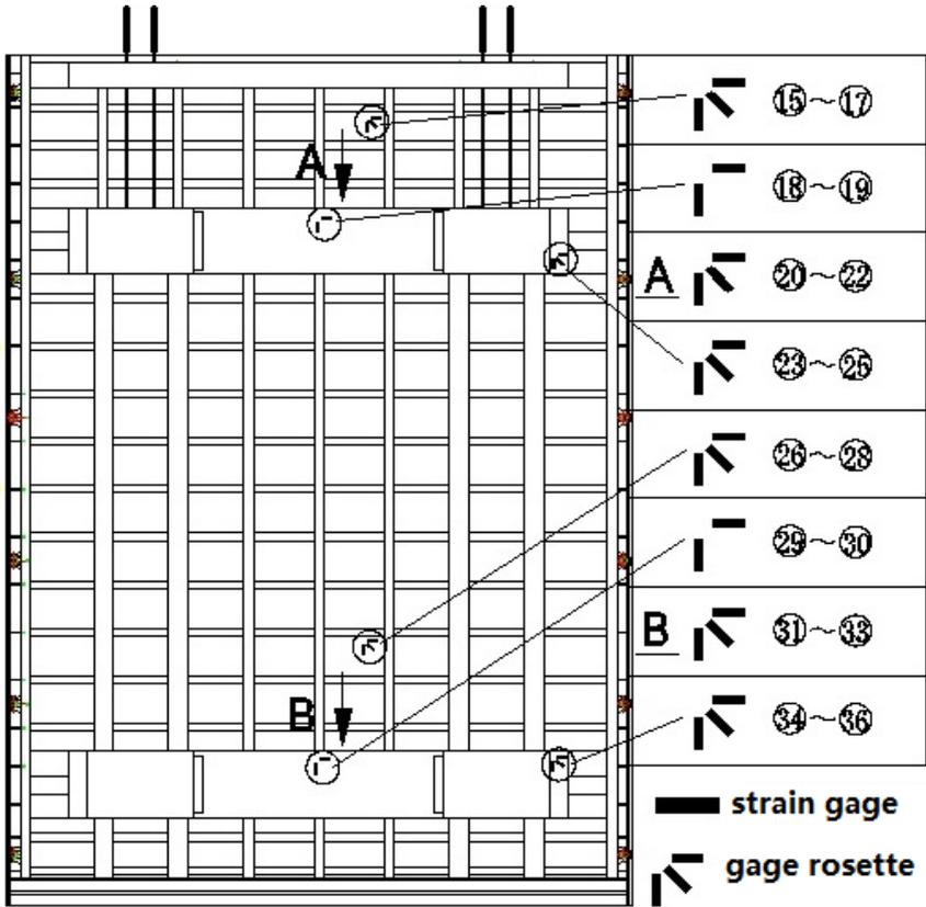
Figure 21. Measurement locations on back surface of arc plate.
