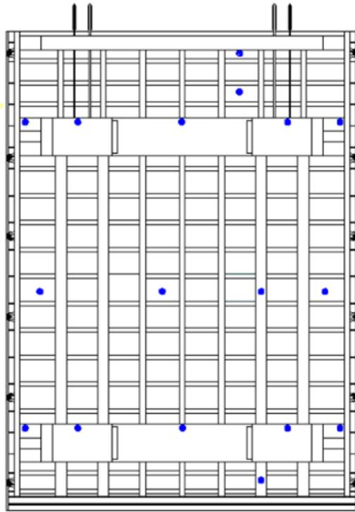
Figure 22. Marking points on the arc plate.
