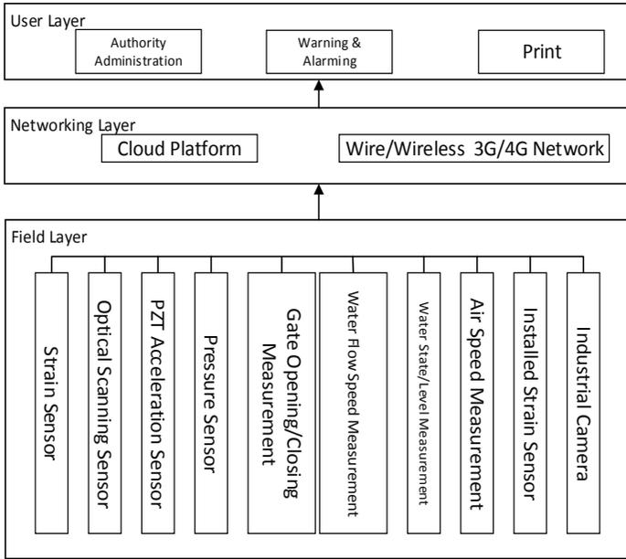
Figure 29. System architecture.
