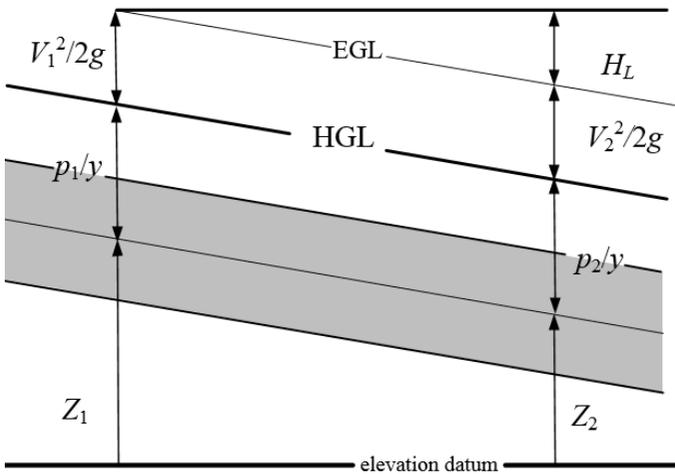
Figure 32. Energy components along pipe with extra energy input.
