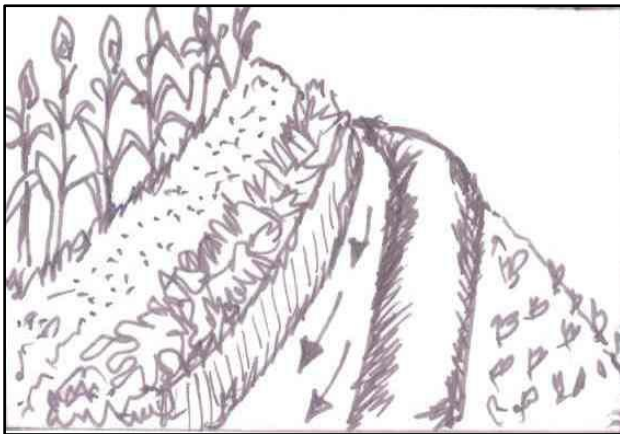
Figure 12. Contour drainage ditch.
