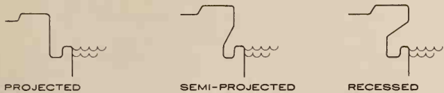
PROJECTED SEMI-PROJECTED RECESSED CONVENTIONAL TYPES OF SCUM GUTTERS
