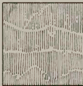
PATENT BUSH-HAMMERED 4-8 cut in 7/8" - for all stones - esp. granite.
