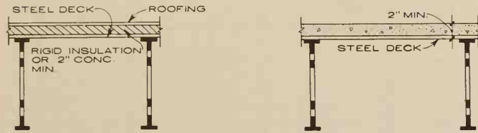
MINIMUM ATTACHMENTS: 2 welds, ea. 1" long or 1/2" bolt or rivet, or 3/16" round steel anchor fastened over beam flange.
