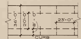
TYPICAL 2-LANE DRIVE - PARALLEL PARKING EACH SIDE
