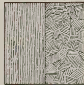
HAND TOOLED Regular or random, for soft stones.
