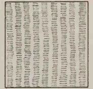
TOOTH CHISELED Soft stones.
