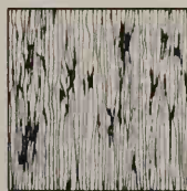
PLUCKED Machine textured for limestone.
