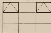
COMBINATION (PROJECTED-FIXED) Alum: No std. by AAMA Steel: Residential No std. sizes by SWI
