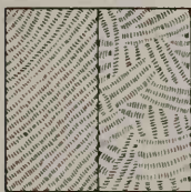
CRANDALLED Regular & random - for soft stones.
