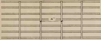
WITH SPACER BARS WELDED 4" O.C.
