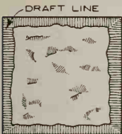
ROCK OR PITCH FACED Rough, "rusticated", for all stones.
