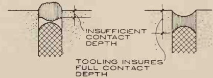
WRONG NOT TOOLED RIGHT TOOLED TOOLING OF BUTT JOINTS
