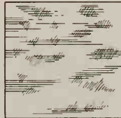
SHOT SAWED Rough, more marked than gang, soft stones.
