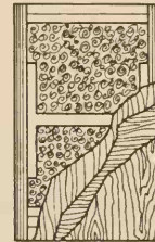
IMPLANTED BLANKS: Spirals or other forms separated or joined, implanted between & supporting outer faces of door.
