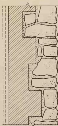
4"-8" STONE BONDED TO UNIT MASONRY BACK-UP; VOIDS SLUSH FILLED; HOLLOW CLAY TILE ALSO USED; NO TIES REQUIRED
