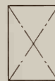
REVERSIBLE WINDOW (SPECIAL) Alum: Architectural No std. sizes by AAMA Steel: No std. by SWI
