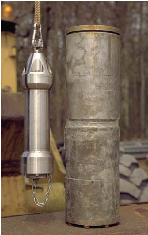
Fig. 63. Tracer Injection Apparatus (TinA, left) and Lycopodium Apparatus (LydiA, right). The diameter of LydiA is 120 mm.
