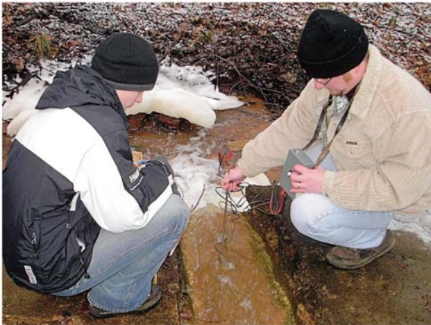
Fig. 52. Flow measurement with an impeller current meter in the discharge channel of a natural lake receiving polluted mine water. The left operator records the time and the right one holds the impeller current meter and the electronic device for counting the turns of the impeller.
