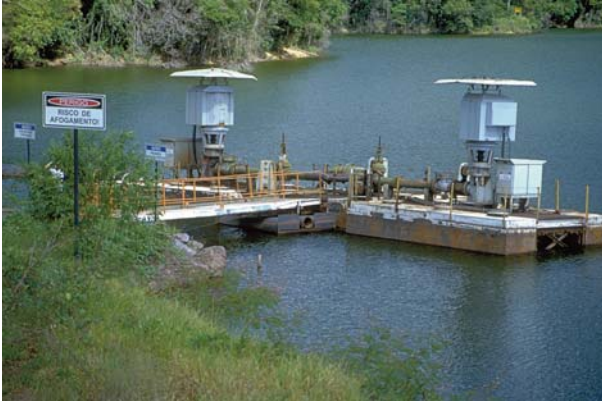
Fig. 31. Settlement lagoon and drainage pumps of an open pit iron mine near Belo Horizonte/Brazil.
