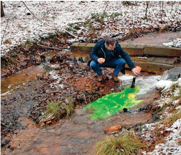
Fig. 48. The Dirac-impulse injection of Na-fluorescein (dark red when it flows out of the bottle, lighter greenish to yellow in colour when it mixes with the stream water) used to measure flow at the inlet of a lake that receives polluted mine water (photograph by Andrea Berger).
