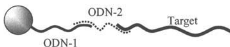
FIG. 6 Schematic illustration of specific capture of nucleic acid fragment by a double-hybridization process onto magnetic polymer particles. ODN-1 oligonucleotide (of a given sequence); ODN-2 oligonucleotides act as a spacer arm and specific to a given part of ODN-1.
