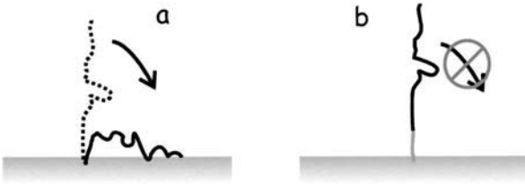
FIG. 8 Glycine tags as spacer sequences. When peptides are attached directly to the surface, additional undesirable interactions might occur (a). The inclusion of several glycine residues at the attachment end is a good strategy to avoid these interactions (b) and usually does not contribute to nonspecific antibody recognition.
