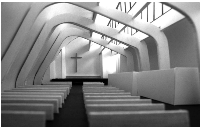
Fig. 15. Riola Church, Bologna, Italy. Alvar Aalto, Architect. 1966. Daylight model study by Jay Adams and Jon Vandervelde. Summer solstice 9 am. Daylight factor = 12%
