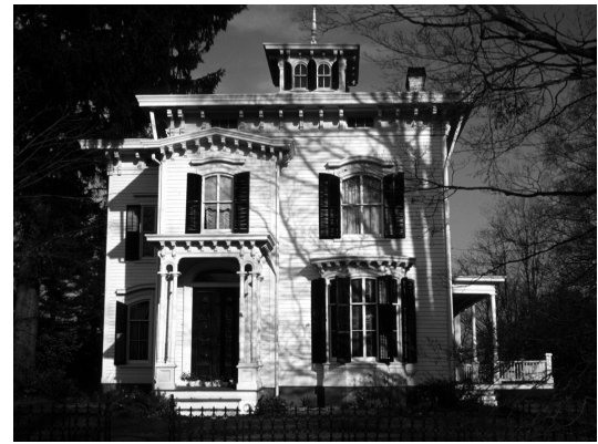
Natural ventilation with porches, extended wings, adjustable louvers and shutters, attic ventilators (under eaves) and roof monitors.
