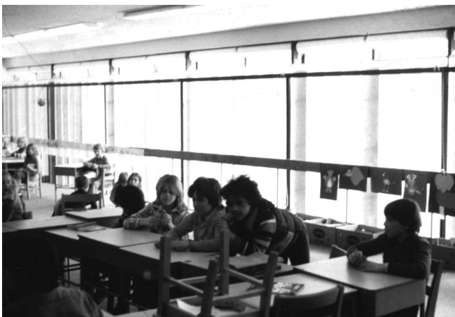
Fig. 10. Elementary School. Athens, VT. Translucent water columns placed in the south window absorbs solar heat while also transmitting daylight. An insulating curtain closes the units at night. John Rogers and George Heller, Architects.
