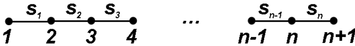
Fig. 1 A path graph tree; S_i is the gossiping matrix when nodes i, i + 1 gossip
