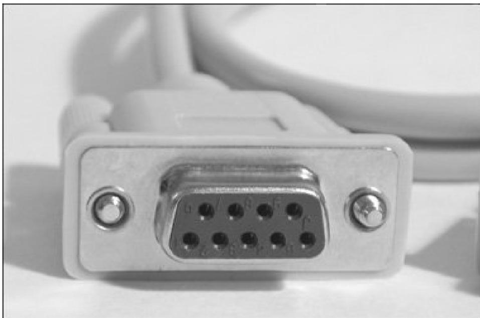
There are usually at least three active pins in a serial cable. They are Rx (receive), Tx (transmit), and Gnd (ground). An example pinout is shown in [Figure 11-6](#). In a DB-9 connector, DCE devices use pin 2 for Rx, pin 3 for Tx, and pin 5 for Gnd, and DTE devices use pin 3 for Rx, pin 2 for Tx, and pin 5 for Gnd.
