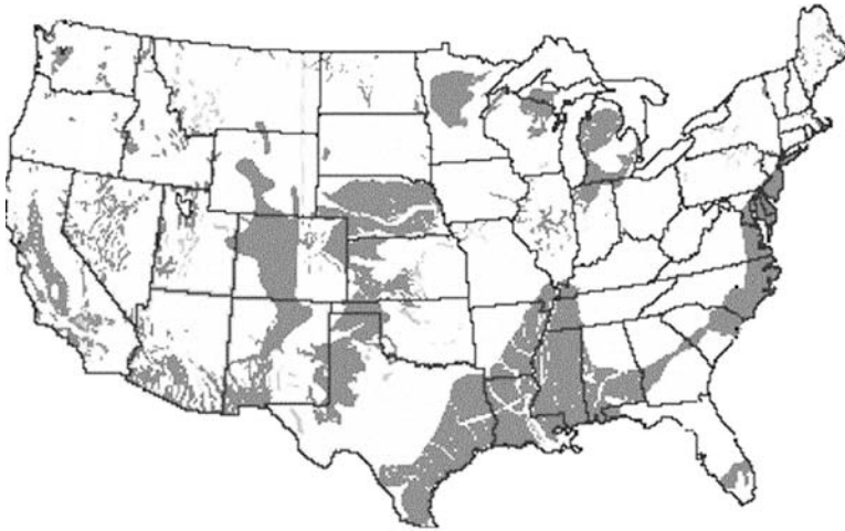
FIGURE 3.54 United States land areas affected by subsidence from pumping groundwater.
