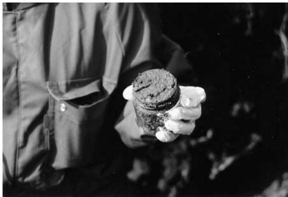
FIGURE 4.15 Filled 250 mL glass sample container of soil. (Photo by Daniel T. Rogers.)
