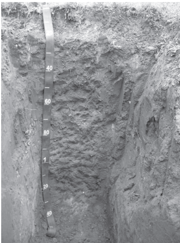
FIGURE 2.10 Montebello Series found in La Verne, CA. Contact of the human-transported material with the natural substratum is observed at 110 cm. Evidence of transported materials includes a thin layer of construction gravels on the left sidewall at 70 cm. The natural substratum is an intact, truncated argillic horizon. (Photo courtesy of Randy Riddle, USDA-NRCS, 2014.)
