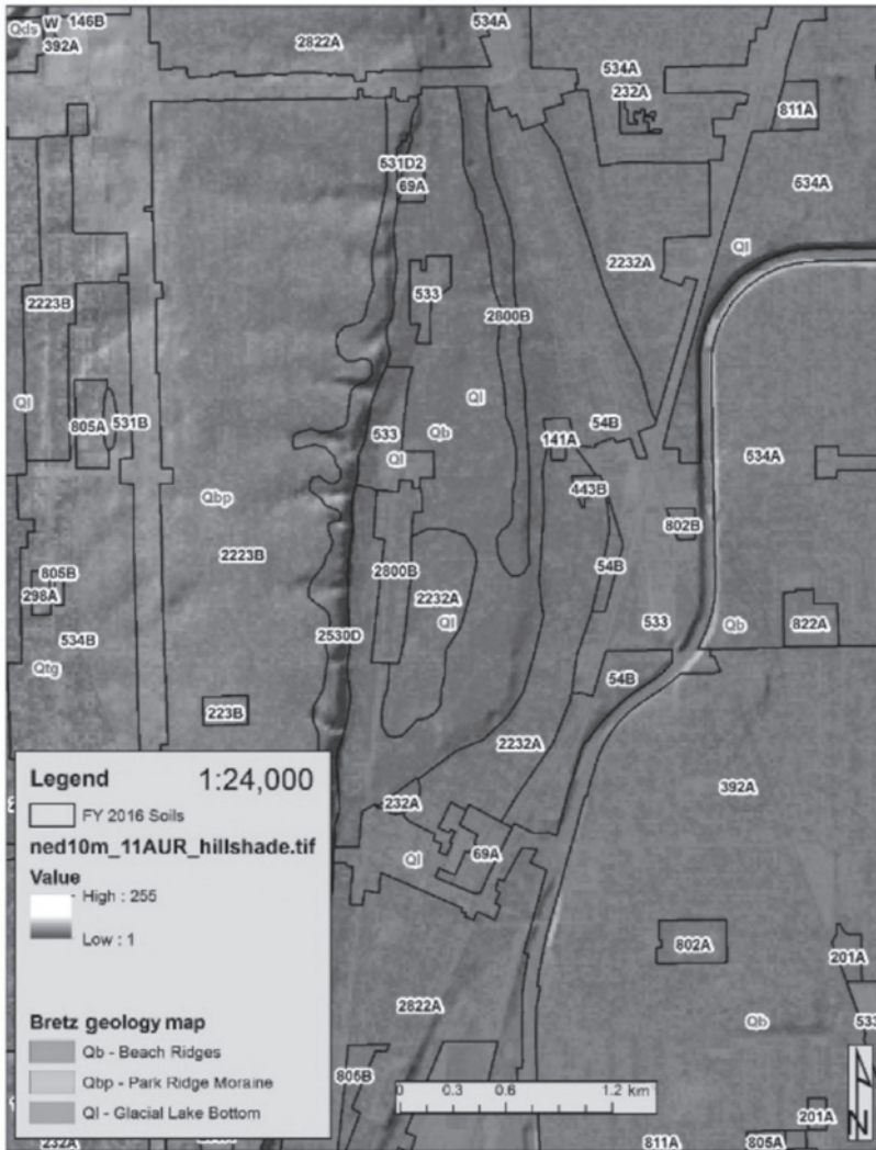
FIGURE 2.5 Chicago and Cook County soil survey–Blue Island Quarter Quad; 10-m DEM and surficial geology (Bretz) maps draped over 2005 aerial imagery. (Map prepared by Kristine Ryan, USDA-NRCS, 2016.)
