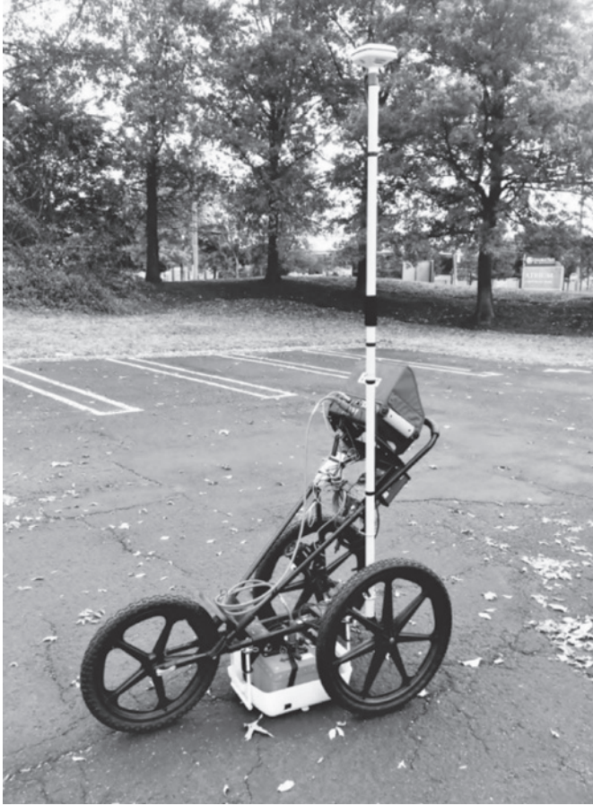
FIGURE 2.19 Ground-penetrating radar (GPR) unit with a 900-MHz antenna mounted in a utility cart with integrated survey wheel and GPR unit. (Photo courtesy of Edwin Muniz, USDA-NRCS.)
