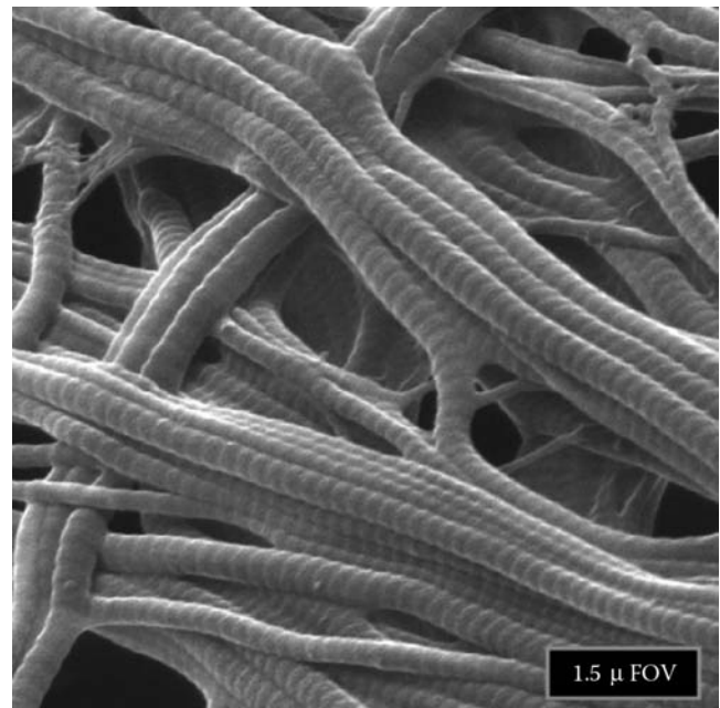
FIGURE 39.13 The complex weave of collagen fibers is shown at a high-magnification [1 \mu\text{m} field-of-view (FOV)] SE image. Note how the edges are brighter, making the three-dimensional nature of the specimen easy to recognize. (Sample provided by NMI Stuttgart.)
