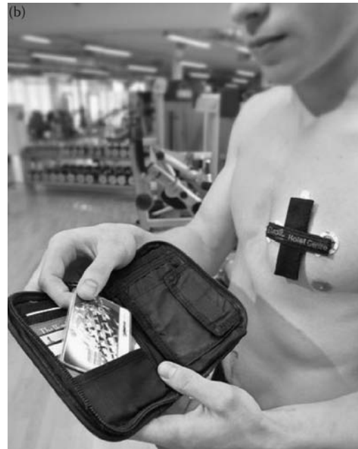
FIGURE 6.1 Wearable vital signs monitor. (a) Monitor for heart rate and other vital parameters. (Courtesy IMEC, Leuven, Belgium and its associated lab at Ghent University.) (b) Patch applied to the body with a wireless data logger kept in the wallet. (Courtesy IMEC, Leuven, Belgium, and the HOLST Centre, Eindhoven, the Netherlands.)
