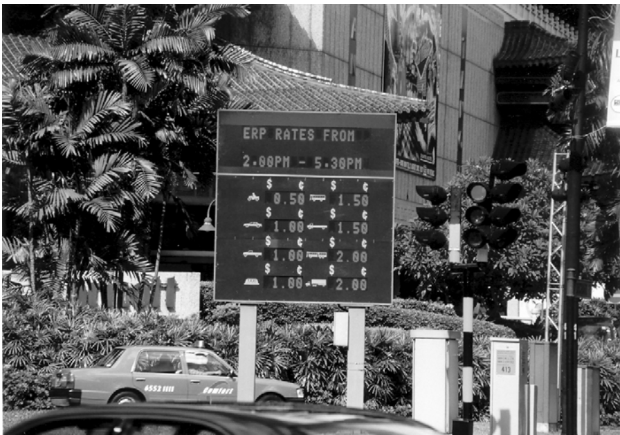
Figure 4.7 The charge display board for Electronic Road Pricing in Singapore
