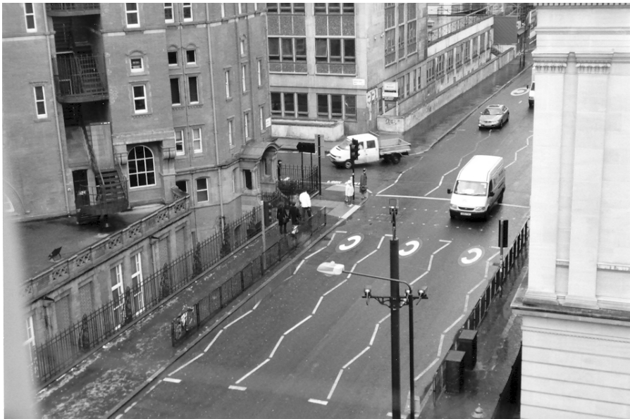
Figure 2.4 Vehicles entering the London Congestion Charging Zone. Note the road markings and gantry with number plate recognition cameras
