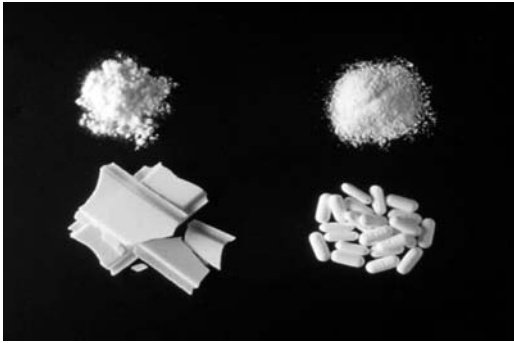
Figure 1 Dry agglomeration processing steps; API powder ( upper left ), compacted API blend ( lower left ), milled and blended compacts ( upper right ), and compressed tablets ( lower right ).
