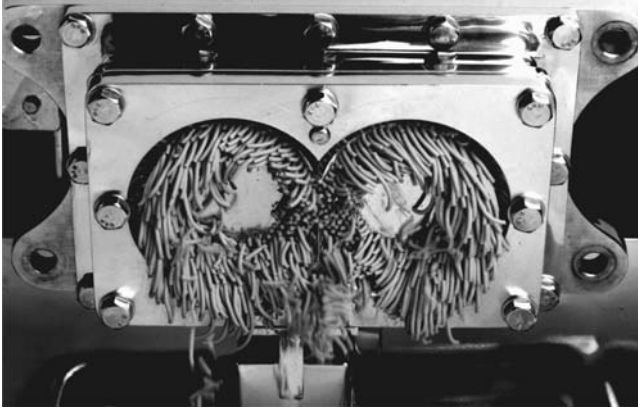
Figure 6 Twin-screw axial extruder. Source: Courtesy of LCI Corporation.
