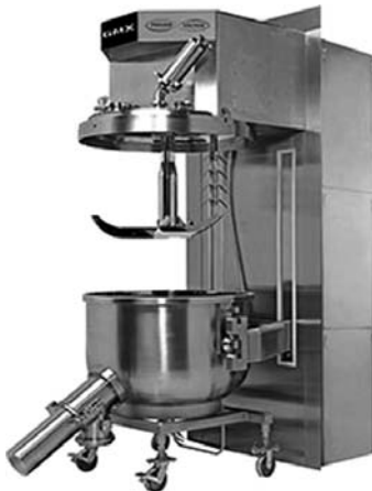
Figure 5 GMX 600 top-drive high-shear granulation/mixing system. Source: Courtesy of Vector Corporation.
