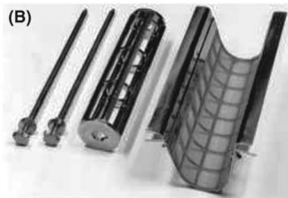
Figure 1 Oscillating granulator: (A) Frewitt MF Line and (B) rotor, screen, and tensoning spindles.
