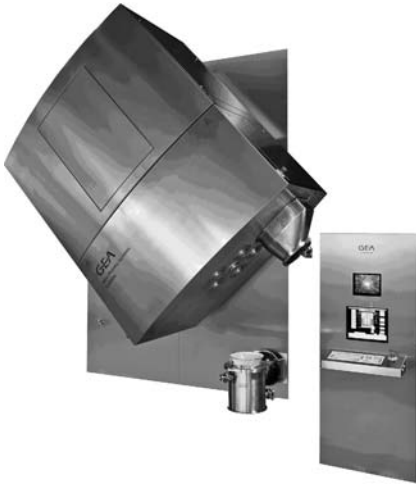
Figure 10 Single-pot high-shear mixer granulator with vacuum drying capabilities UltimaPro™ 600 swinging bowl. Source: Courtesy of GEA.
