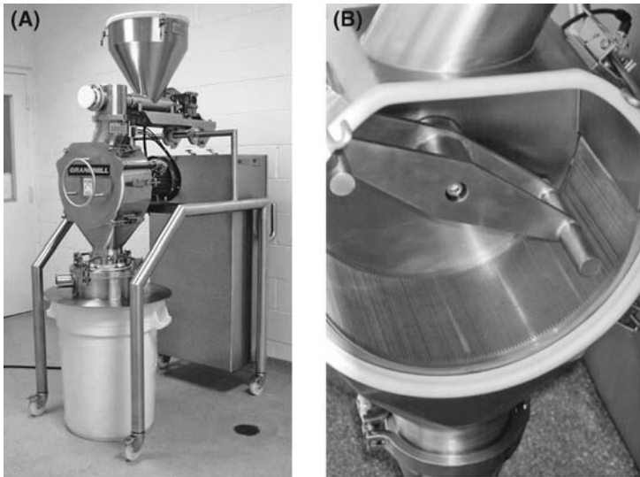
Figure 10 Hybrid design: (A) Granumill, and (B) detail of Granumill rotor and screen. Source: Courtesy of Fluid Air Inc.
