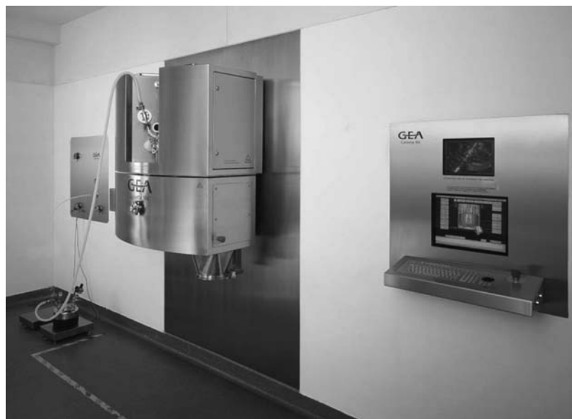
Figure 1 Ultimapro™ 75 microwave/vacuum single-pot processor with swinging bowl. Source: Courtesy of GEA Pharma Systems nv, Wommelgem, Belgium.
