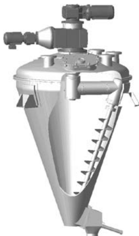
Figure 2 Conical (orbiting) screw mixer.
