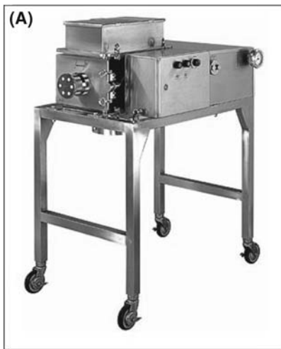
Figure 1 Oscillating granulator: (A) Frewitt MF Line and (B) rotor, screen, and tensoning spindles.
