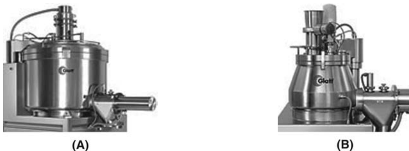
Figure 7 (A) Glatt high-shear mixer VG 1200 with cylindrical working vessel for nonsticky products. (B) Glatt high-shear mixer VG 100 with conical working vessel for sticky products. Source: Courtesy of Glatt GmbH Binzen.
