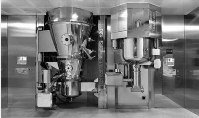
Figure 44 Integrated system showing high shear mixer next to fluid-bed unit. Source: Courtesy of LB Bohle.
