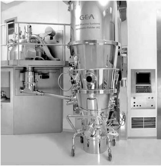
Figure 4 An integrated pharmaceutical manufacturing facility (high-shear granulator–conical-screening mill–fluid-bed drier). Source: Courtesy of Niro Inc.
