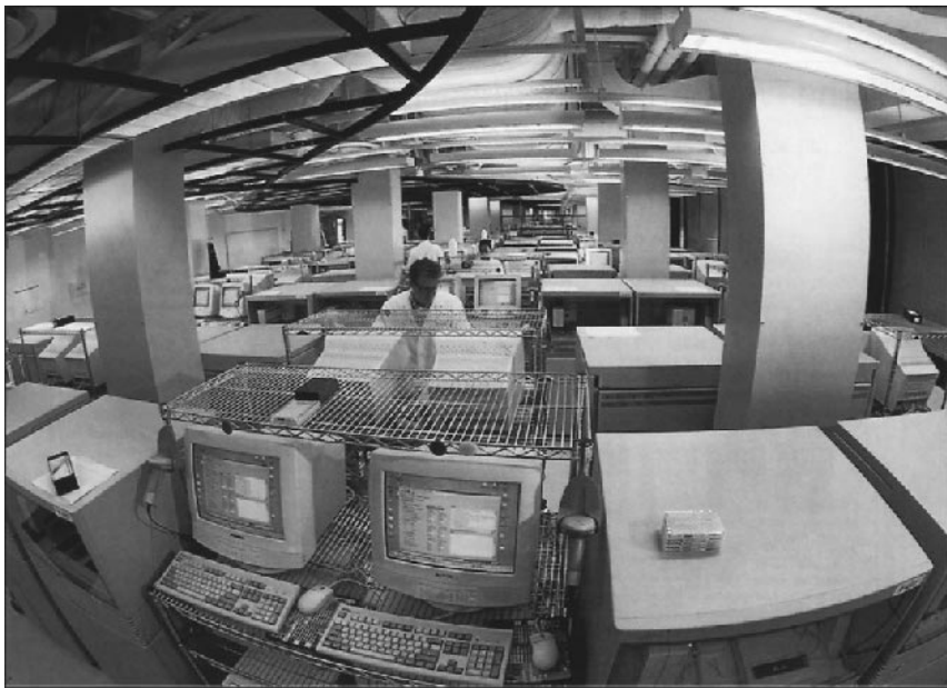
Fig. 16 A partial view of a series of high-throughput DNA sequencers based on multi-capillary-array electrophoresis. (Adapted from Ref. 451.)
