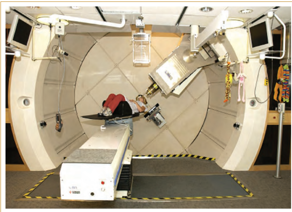
FIG. 24.7. The proton gantry system at the MGH Northeast Proton Therapy Center (MGH-NPTC). An isocentric gantry with a mobile proton beam source is used in conjunction with a robotic patient positioning treatment couch. The robotic unit has six degrees of freedom, three linear and three rotational. The patient is positioned to place the target lesion at the center of beam isocenter.
