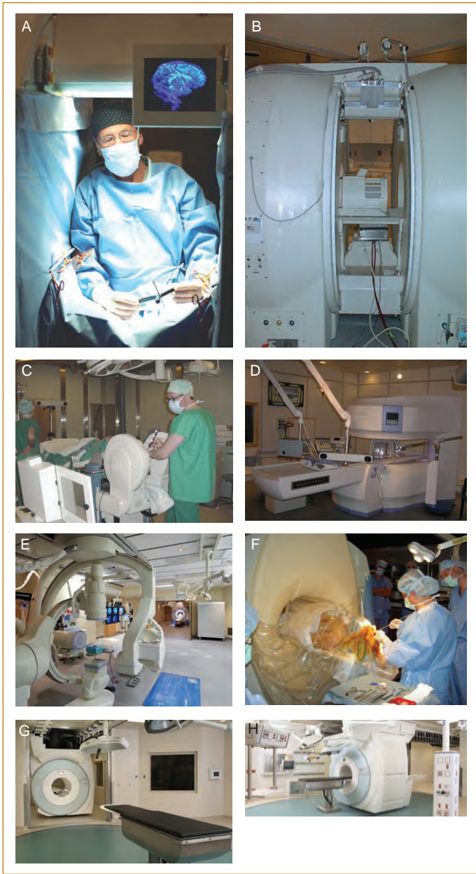
FIG. 22.1. Solutions for MRI-guided neurosurgery. (A) Vertical open superconducting 0.5T interventional scanner with integrated optical tracking system for neuronavigation; (B) same system shown with integrated fluoro x-ray system (courtesy Rebecca Farhig); (C) portable dedicated low field system (courtesy Med-tronics); (D) horizontal open permanent magnet low field system (courtesy Roberto Blanco); (E) two room suite with closed bore 3T scanner and bi-plane fluoro x-ray system (courtesy Walter Kucharczyk); (F) one room solution with 3T scanner; surgery occurs at the back of the scanner to minimize excursion between surgical location and imaging location; (G,H) mobile 1.5T scanner; subsequent to image acquisition, scanner is moved to garage.
