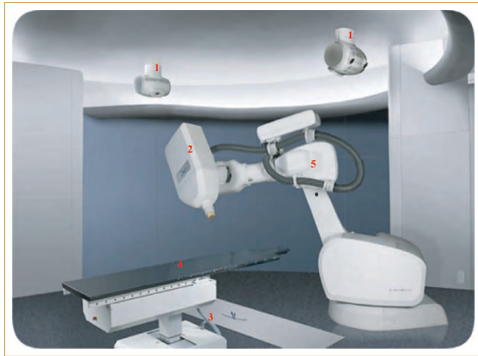
FIG. 24.5. Cyberknife radiosurgery. The CyberKnife device (Accuray™) combines a mobile linear accelerator with image-guided robotic system. During the treatment, patient movement is monitored with minimal time lag by the system's low-dose x-ray cameras. These planar images are compared to digitally reconstructed radiographs derived from the pretreatment CT scan. Based on calculations derived from these comparisons, the computer-controlled robotic arm maneuvers the mobile linear accelerator in response to any changes in patient position during treatment. 1: Diagnostic x-ray tubes; 2: mobile LINAC; 3: camera; 4: couch; 5: robotic arm.
