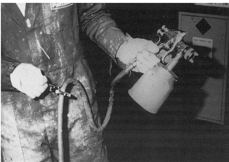
Figure 47.17. Paint sprayer at full-time work, using a plier attachment.
