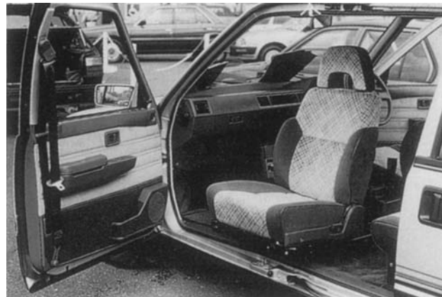
Figure 17.4. A rotating car seat may assist transfers into and out of the vehicle.
