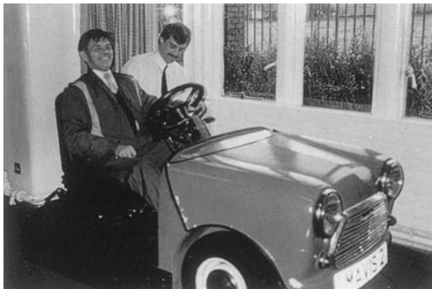
Figure 17.6. A static test unit is used for assessing brake reaction times, brake pressure readings, and steering ability.
