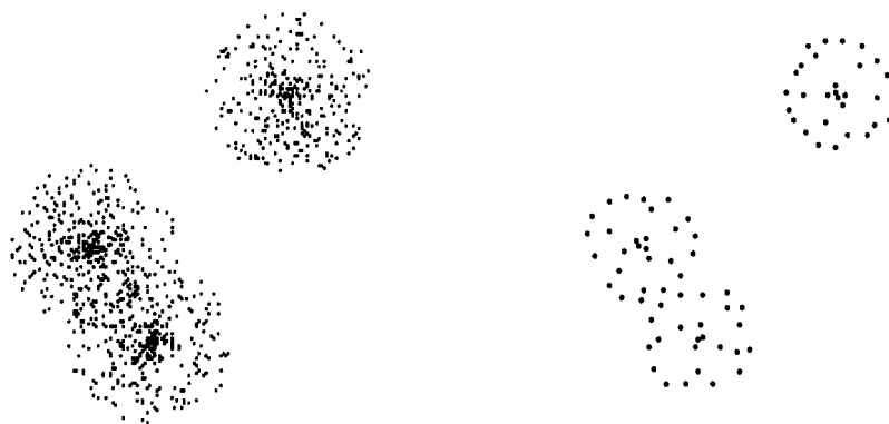
Figure C2.1.10. Input distribution formed by three Gaussian functions in two dimensions, and the corresponding neuron locations after convergence of the neural-gas algorithm.
