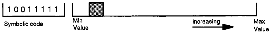
Figure B4.8.3. Two-field state vector with 'symbolic' field and sliding analog field (after Anderson (1995)).
