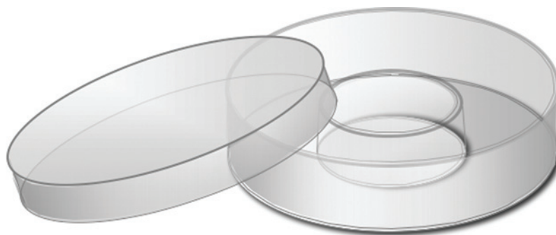
FIGURE 21.4 Sixty millimeter organ culture dish with 10 mm center well.
