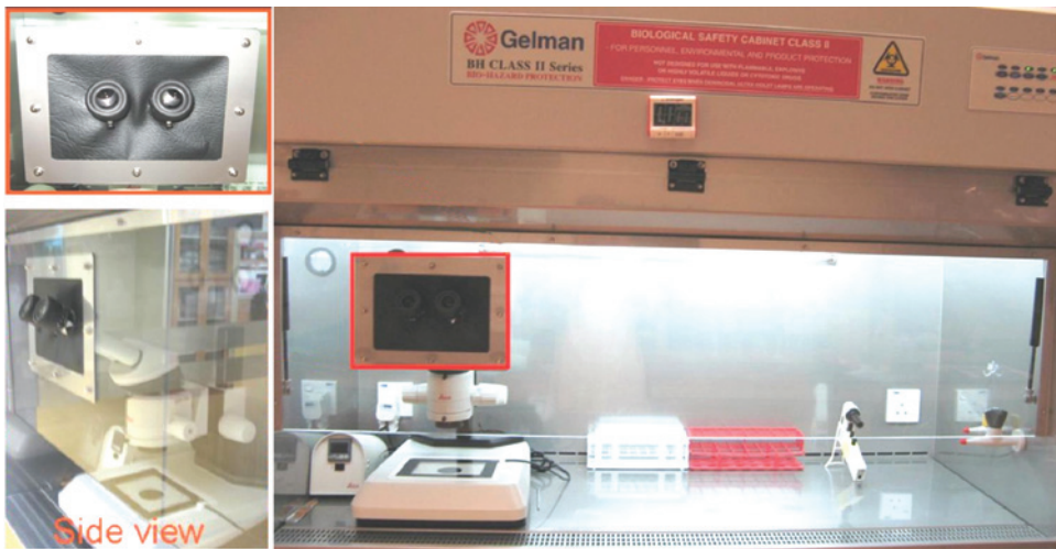
FIGURE 26.6 Biological safety cabinet with fitted dissecting microscope.
