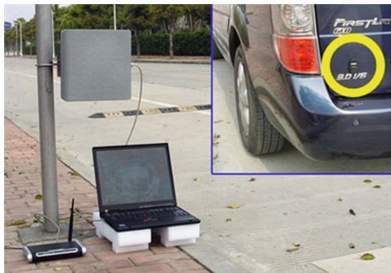
Fig. 5.10 A local node with a RFID reader and a wireless AP; the highlight area in the inset shows an active RFID tag attached to a vehicle
