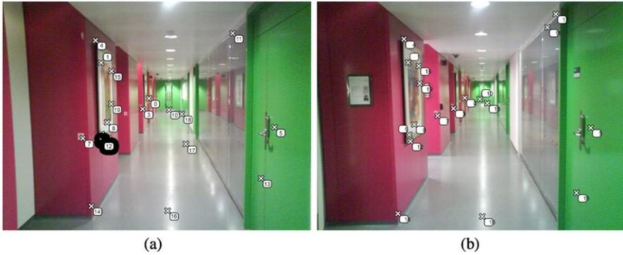
**Fig. 12.13** Localization within a scene with repetitive visual features. Scenes (a) and (b) are captured from different locations in the environment, however, many features in both images indicate a match; scene association is not useful in all situations as most of the matches shown are incorrect
