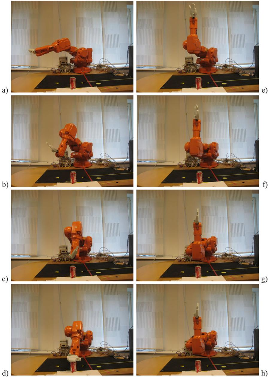
**Fig. 1.12** A trajectory generated from two different randomly initial position reaching for the same object. *In the left column (a)–(d), a successful reaching motion is generated where the final position is on top of the can. The right column (e)–(h) shows a case where the robot reaches an unreachable joint configuration and cannot move along the trajectory*
