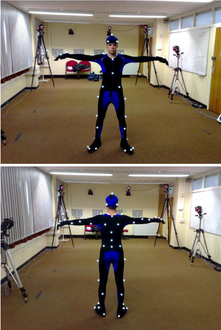
**Fig. 5.9** Optical markers placement—front and back view
