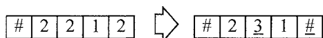
Fig. 5.2. Illustration of the mutation operation in the Michigan-style fuzzy GBML algorithm. This mutation is also used in the Pittsburgh-style fuzzy GBML algorithm
