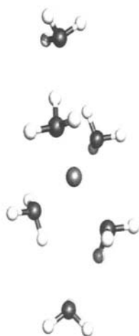
Fig. 8. Lowest energy SCF-MI optimized structure of the complex of the \text{Li}^+ cation with six ammonia molecules
