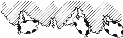
Figure 21 Schematic illustration of the effect of concentration of an immobilized affinity ligand and uneven surface of a solid carrier on specific and nonspecific sorption.
