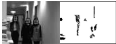
Fig. 4 Three girls walking under a noisy environment. (a) Tracking result. (b) Skin region extraction under bad lighting condition.
