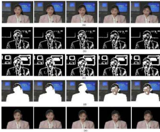
Fig. 6. Semantic object generation results: (a) original images; (b) corresponding luminance edges; (c) color edges; (d) objects obtained by ratio-based method; (e) refined objects.
