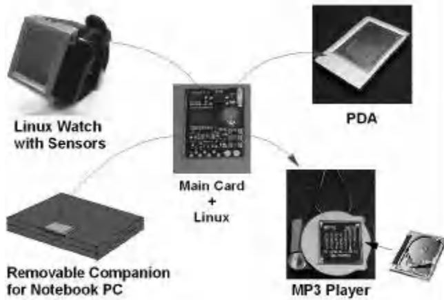
Fig. 3. Modular Concept: Design Variety for other form factors
