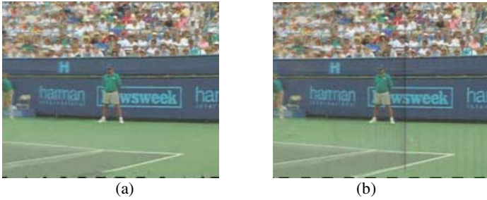
Fig. 7. Sprite coding results for background object sequence Stefan , frame 190, 70kbit/s. (a) Proposed method, and (b) MPEG-4 Video VM
