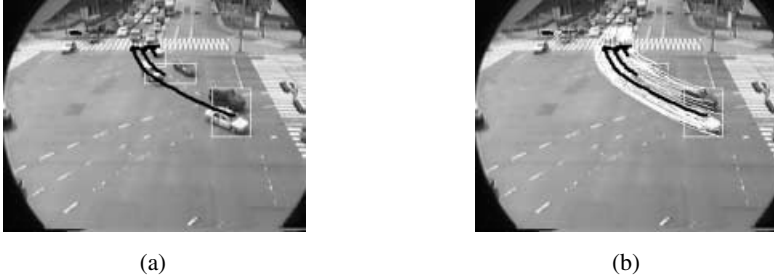
Fig. 4. Tracking results of traffic scene with partial occlusion and neighboring condition by the grouping using only spatial information
