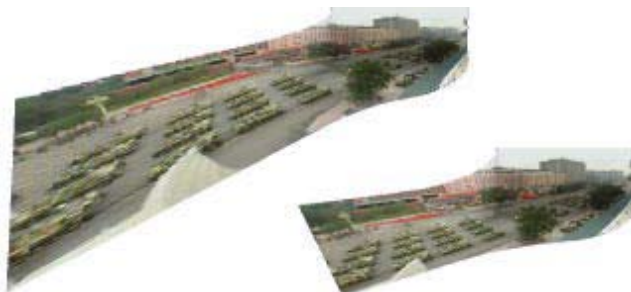
Fig. 2. The upper left mosaic image, size of 1001x1179, is made of 240 frames from a video size of 352x288. Since it is not controlled by local adjustors, the cumulative errors are very serious. The lower right mosaic size of 751x616 is made of the same frames. The cumulative errors are obviously alleviated by using local adjustments.
