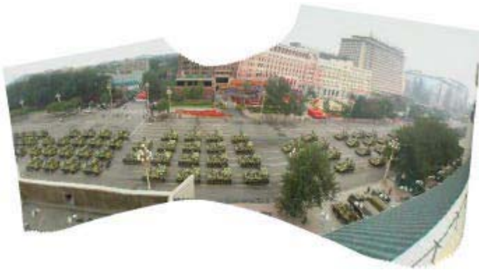
Fig. 3(b) The mosaic panorama made by our double hierarchical algorithm. The pan of the camera is larger than 90^\circ . Its size is 1306 \times 589 .
