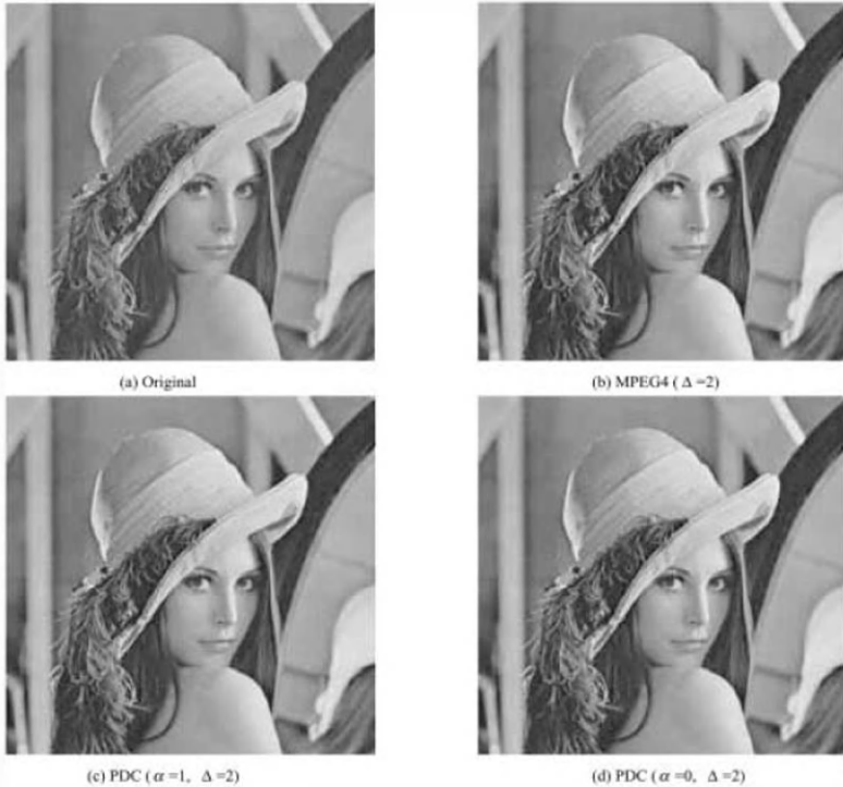
Fig. 4. The reconstructions of the image with the size 512x512 and in grayscale format, named as Lena, through MPEG-4 VTC and the perceptual dithering coding. The quantization step size ( \Delta ) used is 2 and the two weighting values ( \alpha ) are used for perceptually dithering.
