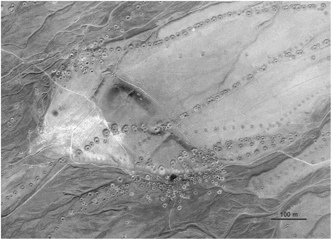
FIGURE 20.8 Clusters of wells at the start of the qanāt line “golan-kariz.” Baharden region, northern piedmonts of Kopet-Dag range. GPS coordinates: N38°23′13.04″ E57°22′49.43″. (satellite image, SAS.Planet.)
