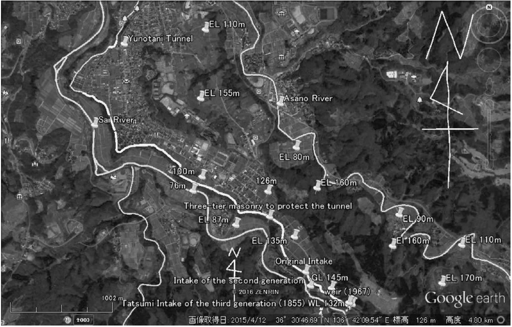
FIGURE 21.4 Alignment of the tunnel on Google Earth shows close location to the scarp of the Otari Terrace. (From HP/Google, Tatsumi Aqueduct, 2015a. With Permission.)
