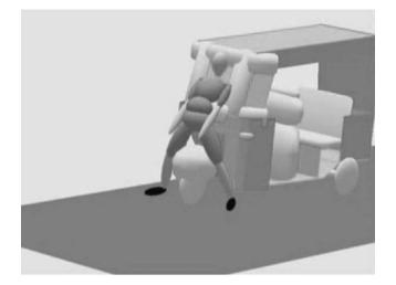
Figure 14.1 A multi-body simulation of a pedestrian to three-wheeler impact to analyze pedestrian kinematics such as head impact speed using a MADYMO multi-body human model (TNO 2012). Courtesy of Sudipto Mukherjee, Indian Institute of Technology, Delhi.
