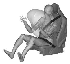
Figure 14.2 A finite element simulation of a frontal crash to analyze the thoracic injury risk for an occupant loaded by seat belt and airbag, here visualizing the shear stress in the ribs with THUMS (TMC 2008). Reprinted from (Mendoza-Vazquez 2014) with permission from Manuel Mendoza-Vazquez.
