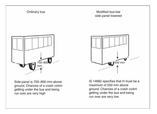
Figure 20.5 Modified bus body showing safe clearance from the ground.
