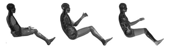
Figure 14.4 Mid-size male models, cut in the sagittal plane to visualize the internal structures: THUMS v3 (TMC 2008), THUMS v4 (Watanabe et al 2011), GHBMC (Vavalle et al 2013).
