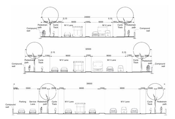
Figure 18.1 Road cross sections for different roads.
