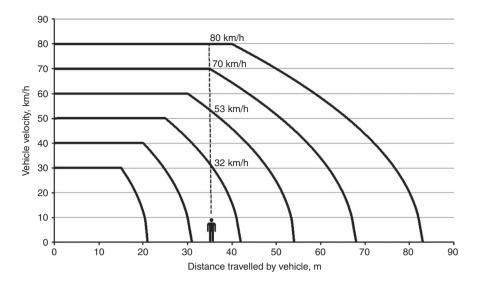
Figure 9.1 Relationship of speed with braking distance for a car on a dry road. Horizontal parts of the lines show the original cruising speed of the car and the curved part shows the braking section (Assumption: driver reaction time: 1.8 s, and average braking deceleration:  $5.8 \text{ m/s}^2$ ).
