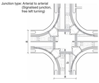
a: Arterial road (24 m to 60 m) b: Length of cycle lane leading upto cycle track (minimum 30 m)
