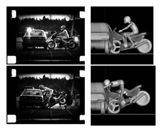
Figure 11.2 Car-motorcycle crash test and simulation.
