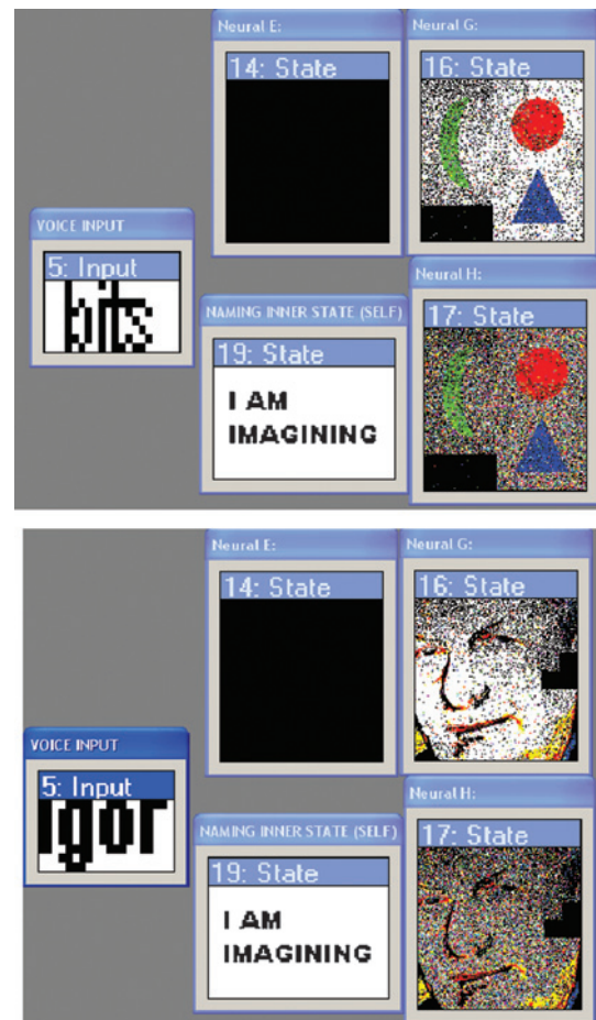
FIGURE A.30 Response of the system to images that represent voice inputs. The memory/imagination module falls into a state which matches the 'voice input'.
