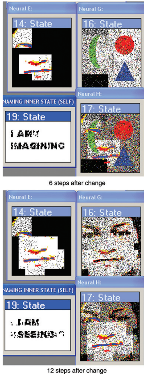
FIGURE A.29 Noticing change in the system. This figure shows the way in which memory of one input lingers while another is being reconstructed and how the 'self' model notices the change.
