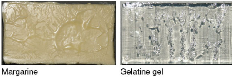
Fig. 9.12 Damage of the cutting surface due to secondary effects caused by ultrasonic excitation of the cutting tool. Absorption heating is responsible for the occurrence of a melted layer on margarine, and a cavitation erosion pattern becomes visible on the surface of gelatin gels
