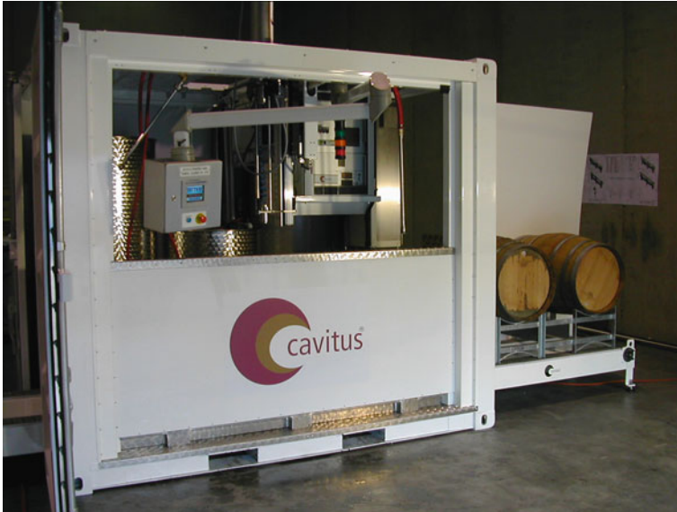
Fig. 24.2 Cavitus' commercial wine barrel cleaning and disinfection system
