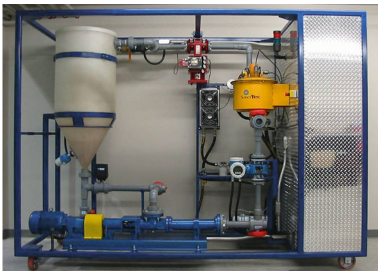
Fig. 7.7 The SonerTec SR-31 5 kW process development sonoreactor system
