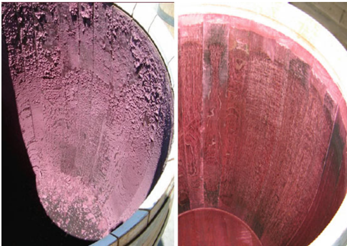
Fig. 24.3 Oak wine barrel before and after ultrasonic cleaning using Cavitus' proprietary ultrasonic cleaning system
