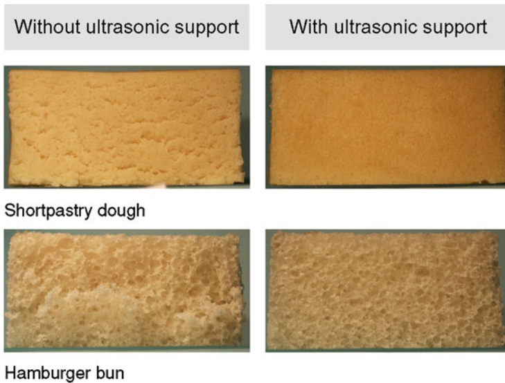
Fig. 9.8 Impact of ultrasonic excitation of the cutting tool on the appearance of cutting surfaces of a compact product (short pastry dough) and a porous food (hamburger bun). Experimental conditions: cutting velocity, 1,000 mm/min; excitation frequency, 40 kHz; ultrasonic amplitude, 12 \mu\text{m}
