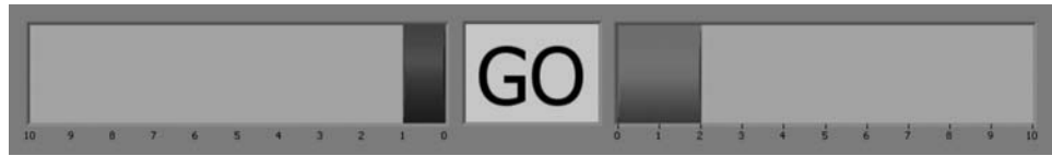
Figure 17.2 Left and right horizontal progress bars. The goal of an interaction experiment is to fill one of the bars, which simulates a real interaction with a robot that needs to reach one side of a room (left or right). The system fills the bars with an error rate of 20 percent; that is, at each step, there was a 20 percent probability that the incorrect progress bar was filled.
