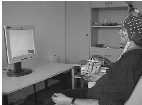
Figure 1.1 The simple game of Pong is revived in a new technological context: imagination of the right hand moves the cursor to the right, imagination of the left hand pushes the cursor to the left. In this manner, the ball that is reflected from the sides of the game field can be hit by the brain-racket. Thus, the user can use his intentions to play “Brain Pong.” Dornhege (2006); Krepki (2004); Krepki et al. (2007).
